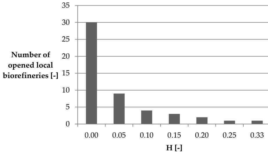
**Figure 9: Number of opened local refineries as a function of H which is the required minimum used fraction of the biorefinery's capacity**
