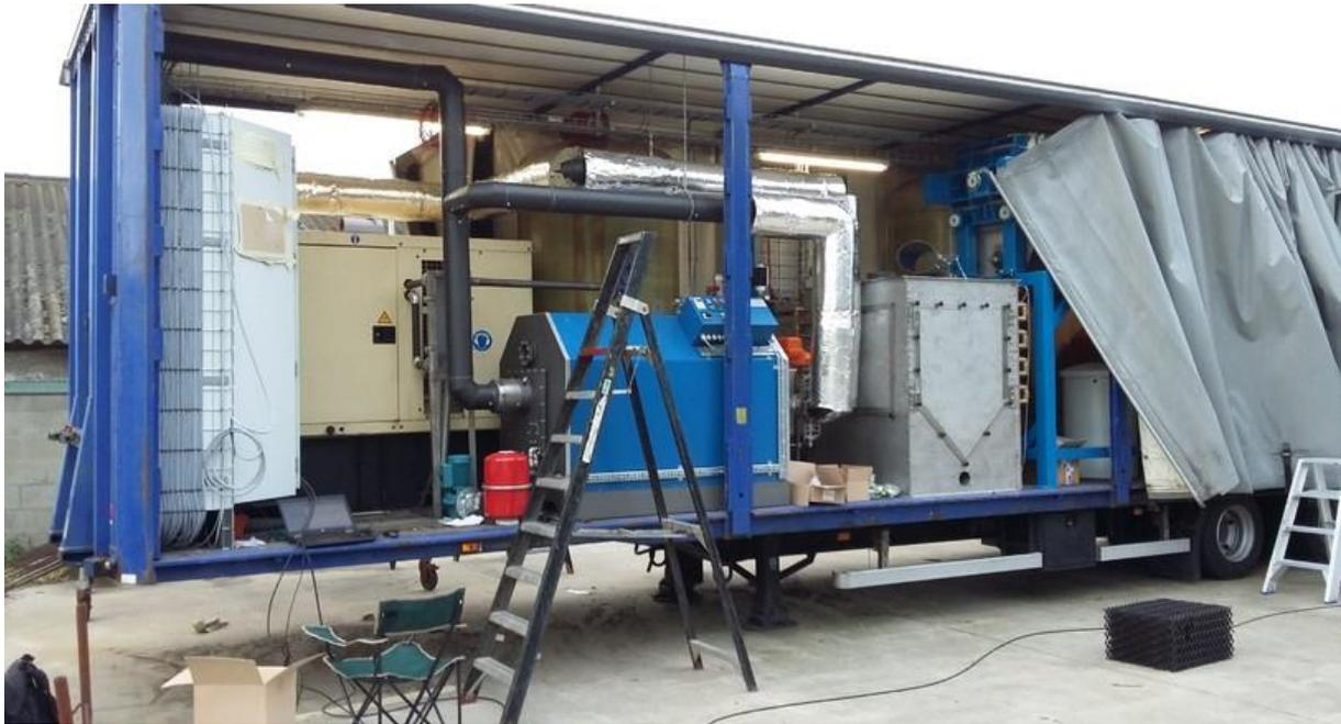
**Figure 4: Grassa! mobile installation for biorefinery; introduced in 2016 (Ingenieur, 2016)**
