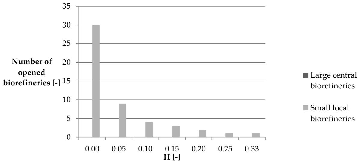
**Figure 11: Ratio between opened large central biorefineries and small local biorefineries against the required minimum used fraction of the capacity at a biorefinery**
