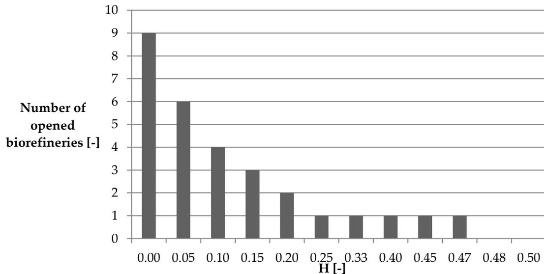
**Figure 7: Number of opened central biorefineries as a function of  $H$  which is the required minimum used fraction of the biorefinery's capacity**
