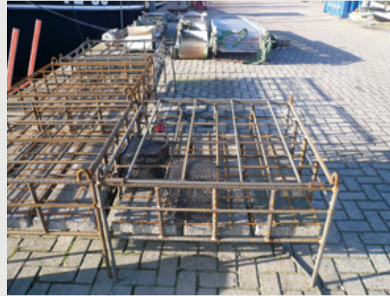
Figure 2: Rack with cages employed in the Voordelta pilots. Shellfish are placed in the PVC cages (small, black), the larger steel racks are intended for physical protection and stability.
