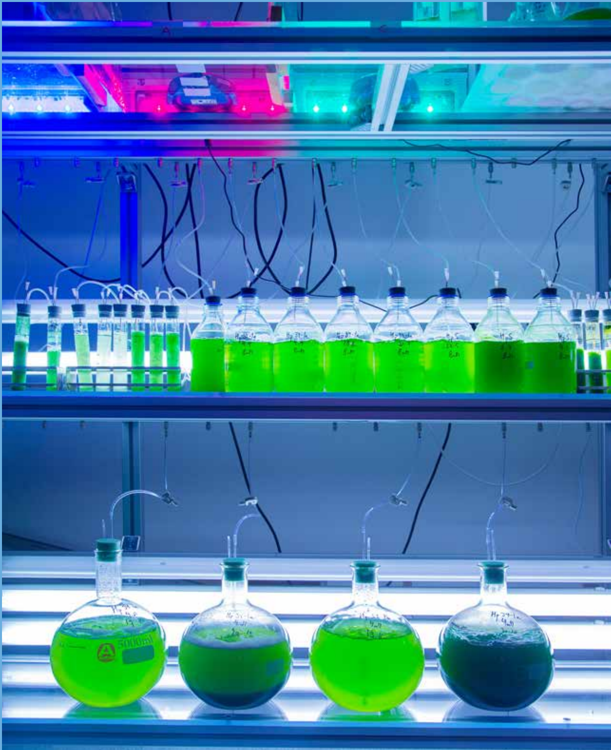
Figure 4.5 Cultivation of different algae strains under artificial (LED) lights.
