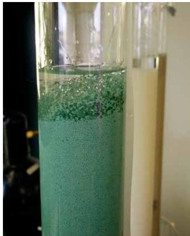
Figuur 7.4. Elution of steviol glycosides from adsorption column.
