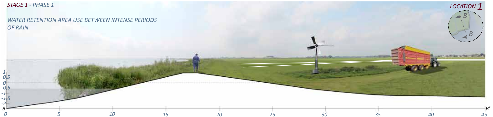
Figure 102 The water retention zone is visible at this image. During dry periods the water pumping station at the area is able to eliminate surplus water. However after periods of extreme rainfall, the retention area can be filled with water out of the polder where
