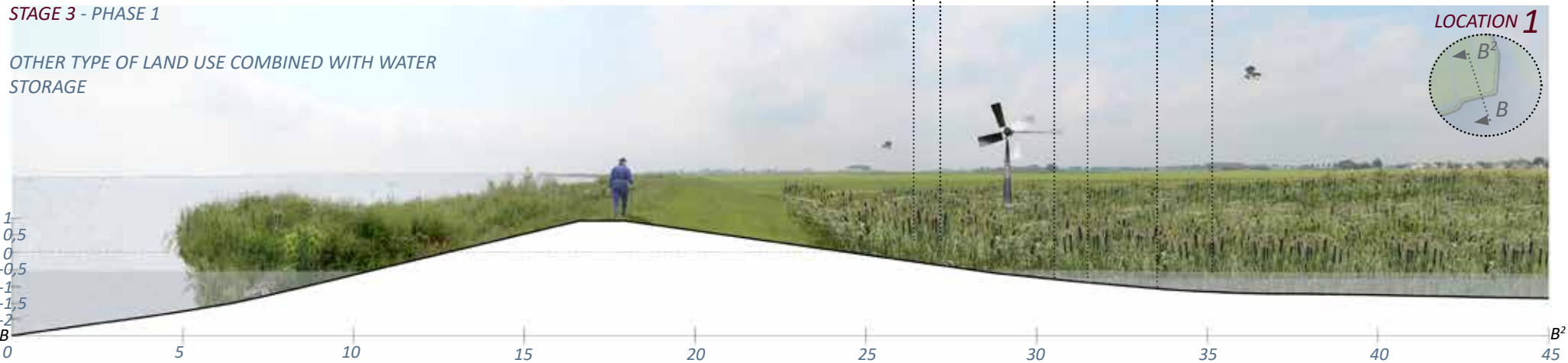
Figure 104 The ideal situation is a permanent rewetted area. This situation will delay the soil subsidence as a result of peat demolition, since oxygen will no longer be able to come into contact with the peat. Also less nutrients will be necessary to fertilize the crops at the wet terrains. Next to this vegetation will be able to purify the water. This combined with a permanent degree of water storage.
