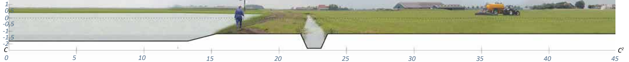
Figure 112 In this illustration it becomes clear how the local retention zone could function. Redundant water from the area can flow into the lower excavated fields. It depends at the capacity of the local water pumping stations how deep such fields must be excavated in order to reduce the water level in nearby ditches. The deeper such excavated fields, the more water they can retain.
