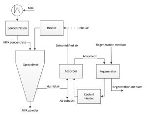
Fig. 1. Schematic representation of a closed-loop dryer for milk powder production. The adsorber can either be the membrane contactor or zeolite system.
