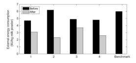
Fig. 6. External energy requirements before and after heat integration.
