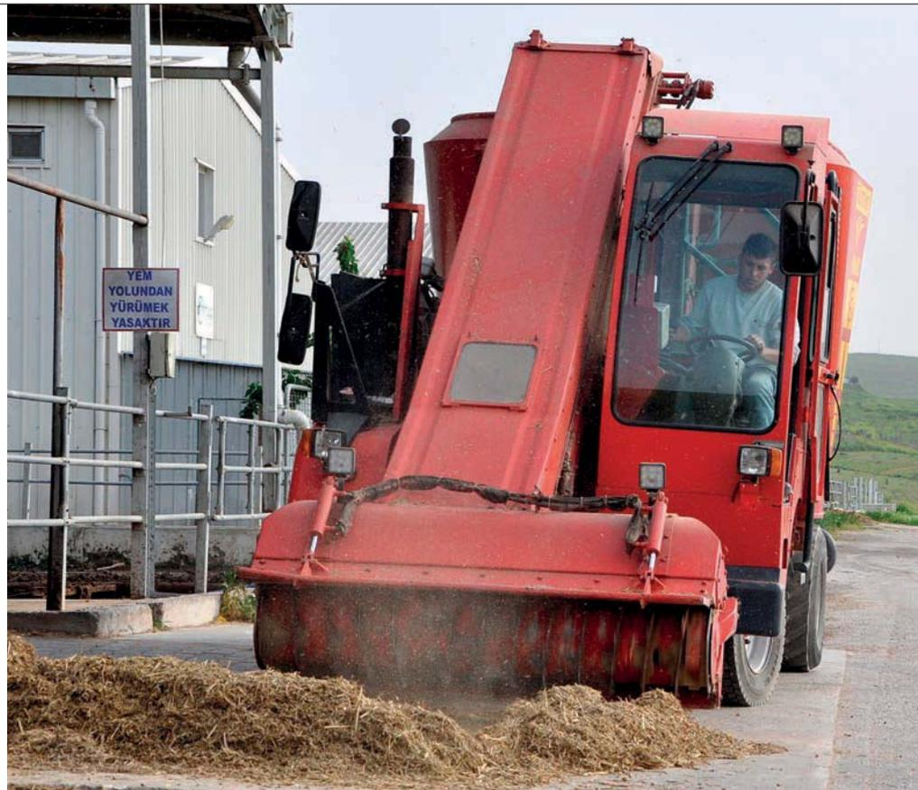
*Above: a self-propelled machine mixes and feeds the herd's TMR*
