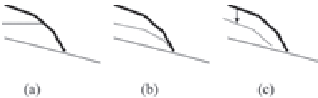
Figure 14: Dredging method; (a) dredge top first, (b) dredge proportional, or (c) dredge uniform.
