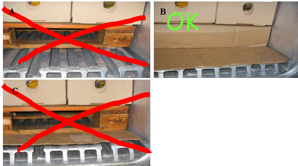
Figure 20. Examples of covering up the T-bar floor (when working with pallets) at the door end to avoid air return through open area (A & C). In the correct picture (B) the pallet and floor is covered, but the T-bars are left open. When working without pallets C is also correct.
