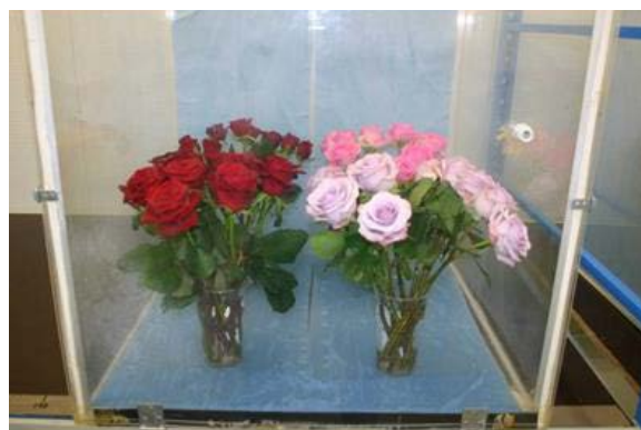
Figure 23. Example of hotboxtest. Condensation on the box hinders the view somewhat.
