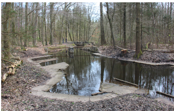
1.7a Physical models in the 'Waterloopbos' (Hydraulics Laboratory): Willemstunnel Rotterdam (schaal horizontaal 1:75, verticaal 1:37.5)
