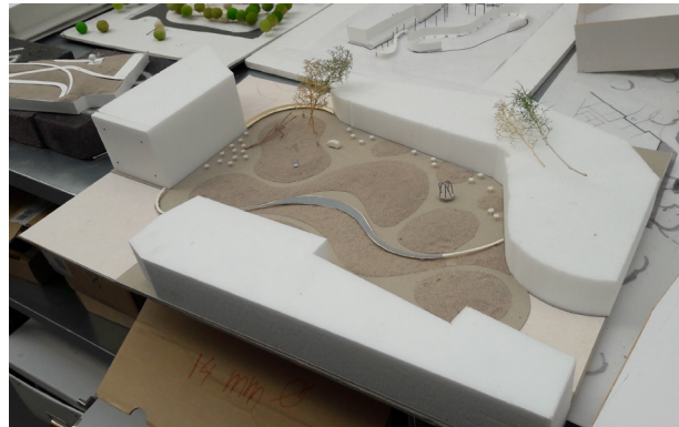
3.29b Example of modelling on different scales in one project: more detailed model to test height of planting areas (sand, foam, cardboard);
