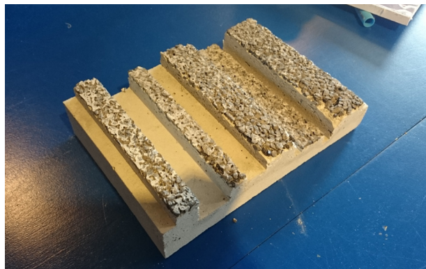
3.8 Example of a 1:1 material test for a sluice wall by ZUS
