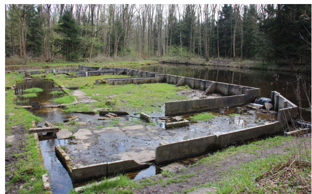
1.7b Physical models in the 'Waterloopbos' (Hydraulics Laboratory): Koelwaterwatervijver Maasvlakte-centrale (scale unknown)
