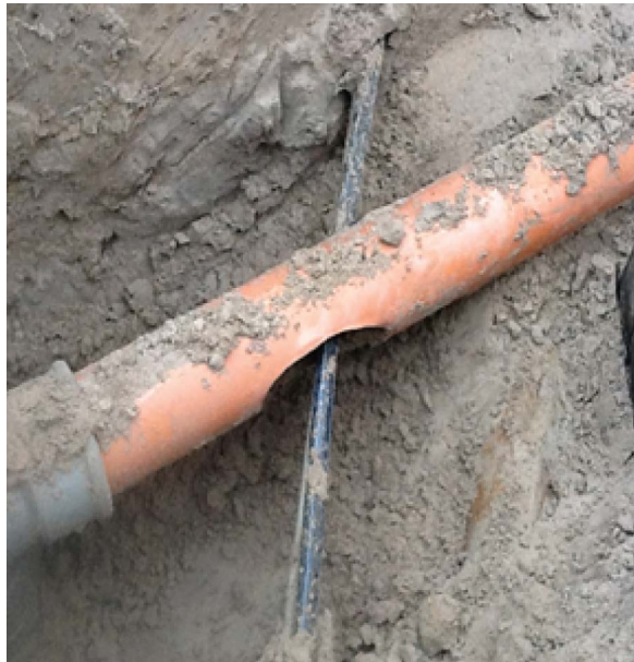
Figure 2.2: Damage to a lateral connection by a cross drill (Langeveld and De Haan, 2014).
