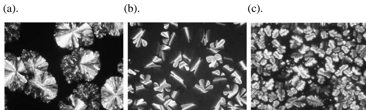
Figure 2. Polarized optical microphotographs of (a) 2-3T1 at 64 °C, (b) 2-3T2 at 63 °C, (c) 2-4T1 at 57 °C, all indicating a Col h phase (See the Appendix at the end of the thesis for the color pictures).
