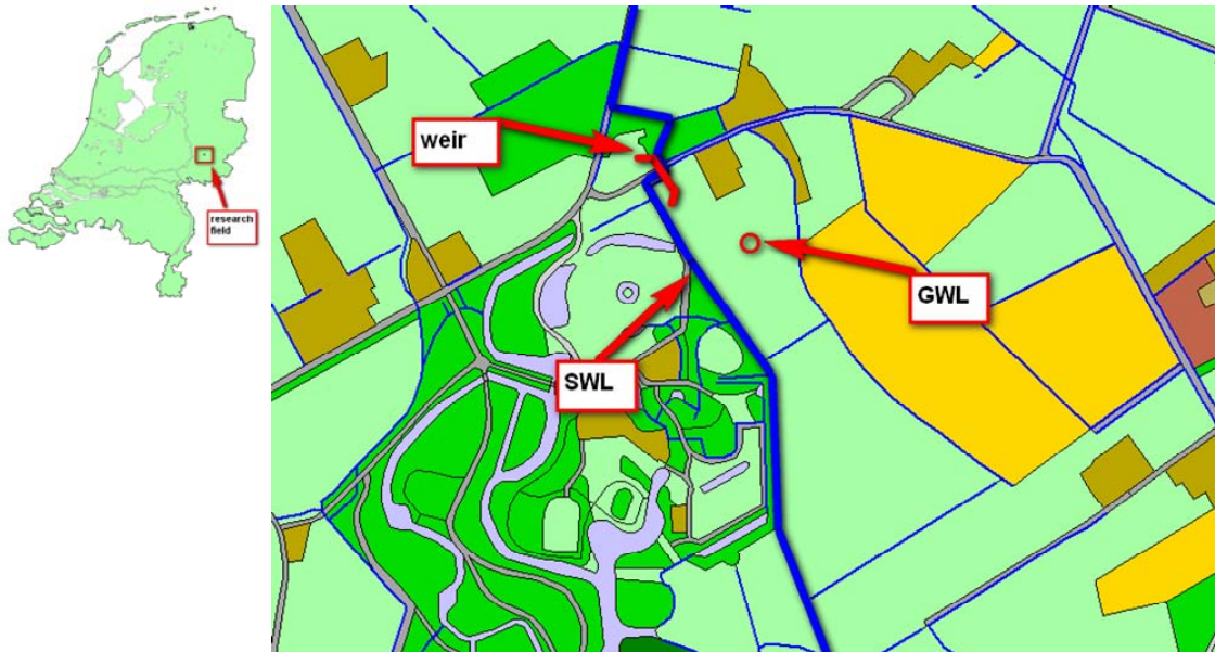
Figure 5.1 Location of monitoring site at the Wildenborch estate where groundwater levels (GWL) and surface water levels (SWL) were measured and controlled by a weir.
