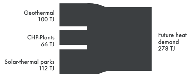
Figure 79: Sankey diagram of the heat balance
