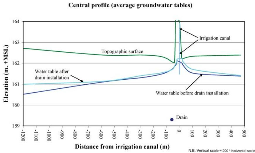
Figure 2. Impact of interceptor drain on long-term average groundwater table.
