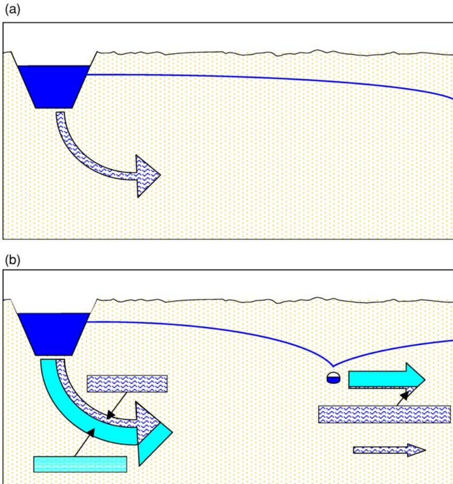
Figure 3. Concepts of induced and net intercepted seepage. (a) Situation before drain installation; (b) Situation after drain installation.
