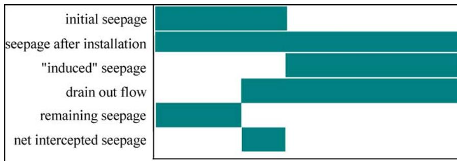
Figure 4. Determination of induced and net intercepted seepage.
