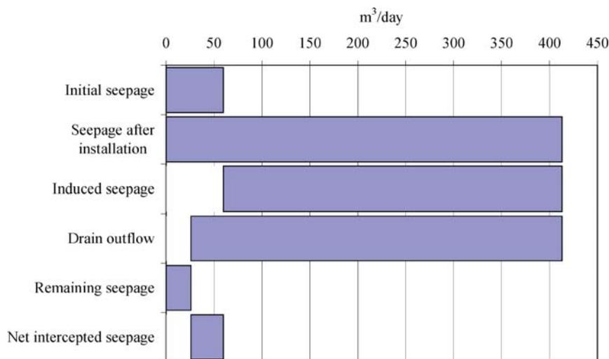
Figure 6. Simulated induced and net intercepted seepage; reference situation. The volumes refer to the canal section adjacent to the interceptor drain (1828 m).
