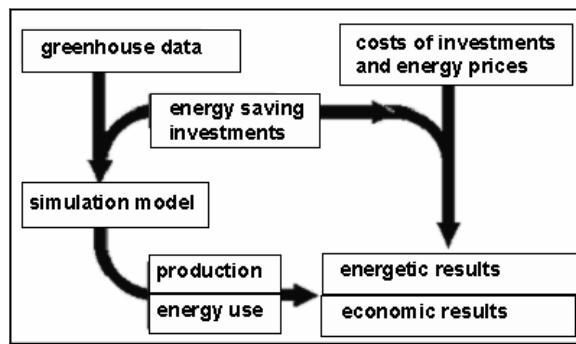
Fig. 1. Schematic overview of EOM. First, users are able to enter their greenhouse data, energy prices and costs for investments. Then they must select one or more energy saving investments. Subsequently the climate model KASPRO will simulate the effect of these investments. Finally the energetic and economic results will be presented.
