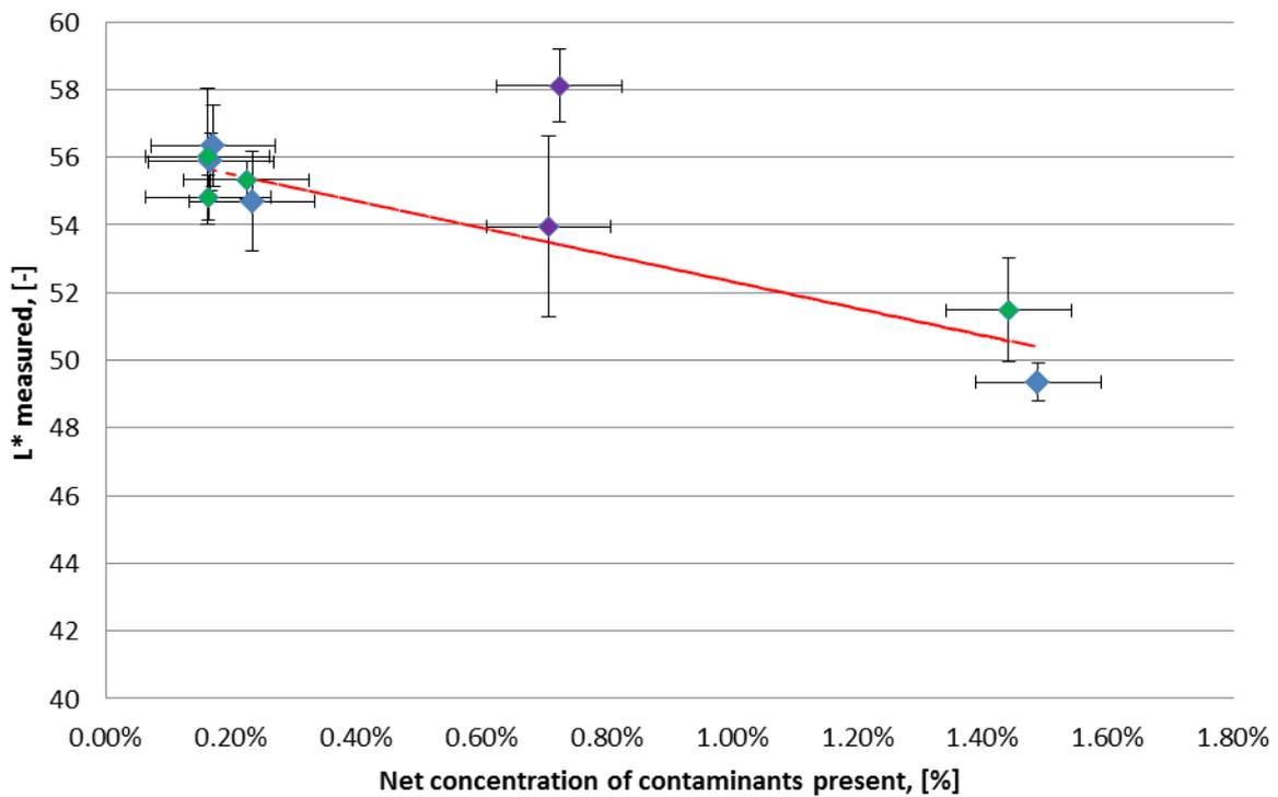
Figure 37: The correlation found between the measured L\* lightness value for the sample of task 3 and the total concentration of contaminants estimated to be present in these samples. The colours indicate the collection systems: purple for deposit-refund systems, green for separate collection systems and blue for mechanical recovery systems.
