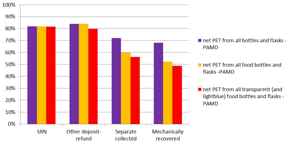
**Figure 12: The net PET material content of sorted PET products originating from three different collection systems in [% w dm/w gross].**
