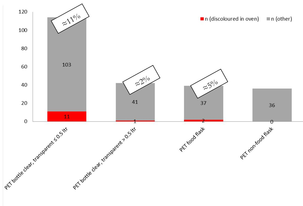
Figure 9: The division of barrier PET bottles over the PET bottle categories. n(other) indicating both the amount of tested bottles that were found not to contain a barrier and non-tested bottles, that could not have a barrier based on the type product they contained (for instance water). Percentages refer to total amount of barrier bottles in the categories, expressed in percentage.
