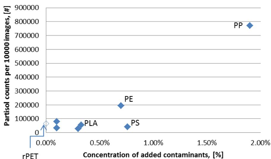
Figure 15: Relationship between the concentration of added contaminants and Particle count.
