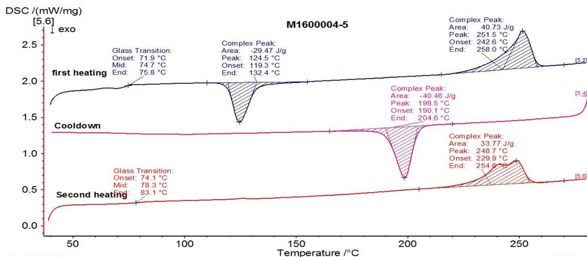
Figure 31: Thermogram of DSC measurements on 4.7 mg of sample 5.
