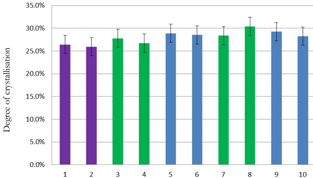
Figure 32: The degree of crystallisation of the 10 types of PET deduced from the melting peak in the second heating run. The colours indicate the collection systems: purple for deposit-refund systems, green for separate collection systems and blue for mechanical recovery systems.
