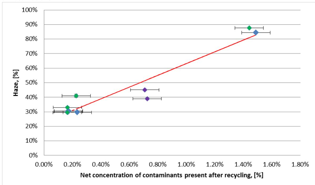
**Figure 36: The correlation found between the measured haze for the samples of task 3 and the total concentration of contaminants estimated to be present in these samples. The colours indicate the collection systems: purple for deposit-refund systems, green for separate collection systems and blue for mechanical recovery systems.**
