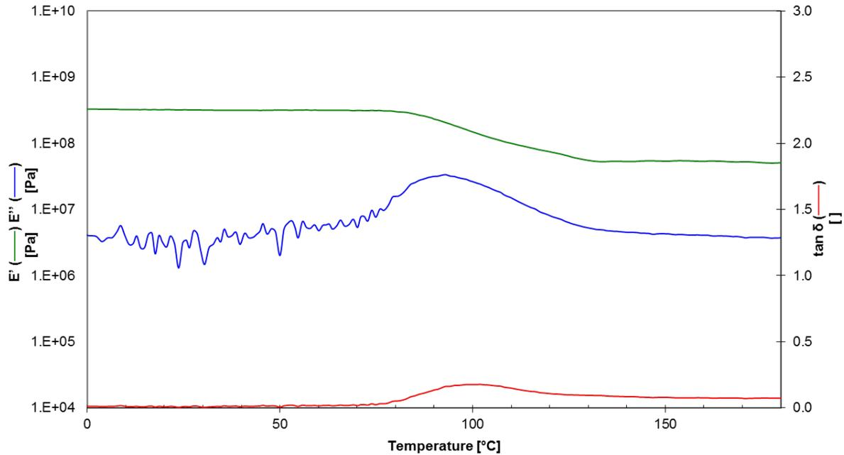
Figure 23: Typical DMTA thermogram of semi-crystalline PET.
