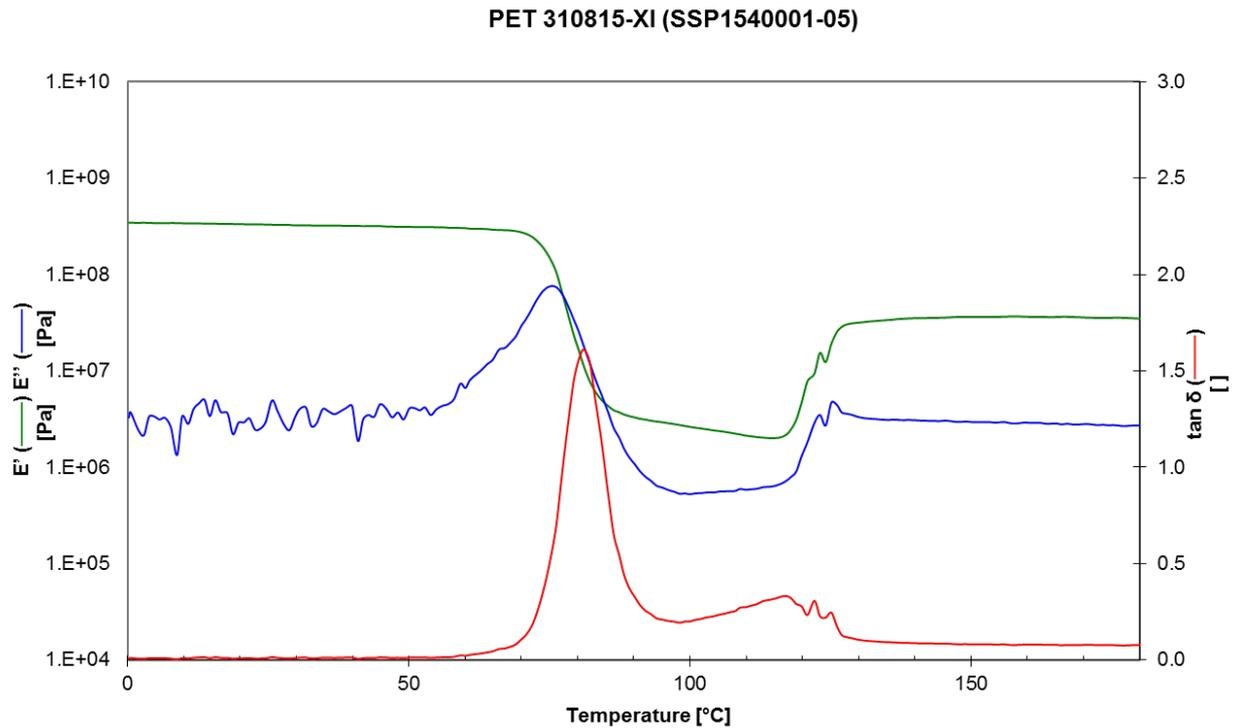
Figure 22: Typical DMTA thermograms of amorphous PET around the glass transition temperature.<sup>19</sup>
