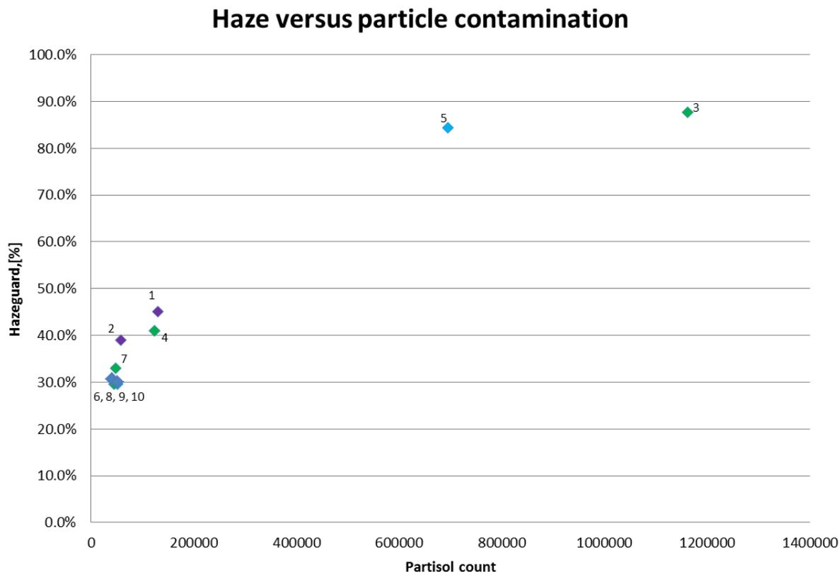
**Figure 29:** The relationship between the particle counts and the determined haze values. The numbers indicate the combinations of feedstock and process studied.
