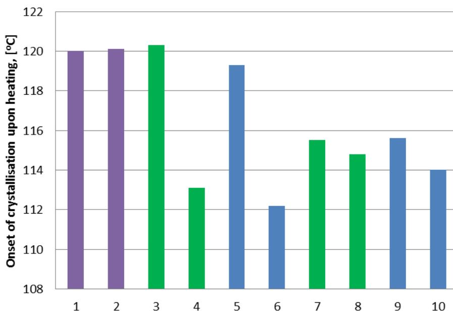
Figure 34: Onset of crystallisation upon heating the rPET, derived from the first heating run [°C]. The colours indicate the collection systems: purple for deposit-refund systems, green for separate collection systems and blue for mechanical recovery systems.
