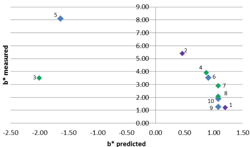
Figure 35: example of modelling b\* with the derived property parameters and the concentrations of contaminants present in the samples of task 3 after recycling. The colours indicate the collection systems: purple for deposit-refund systems, green for separate collection systems and blue for mechanical recovery systems.
