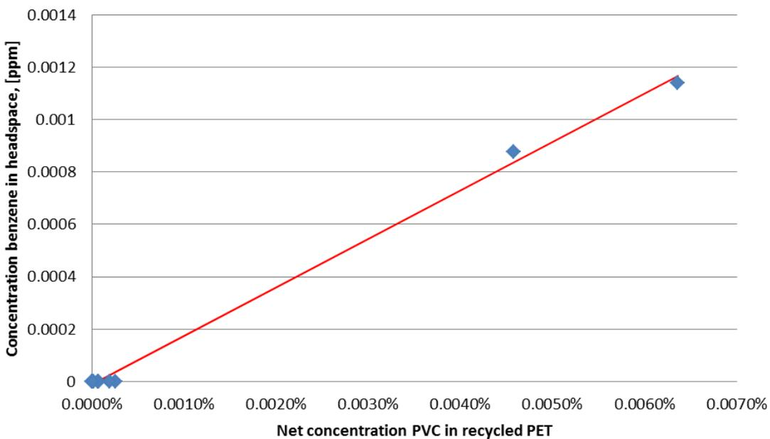
Figure 38: The correlation found between the measured benzene emission values in the headspace after SSP treatment in the samples of task 3 and the estimated concentration of PVC in these samples.
