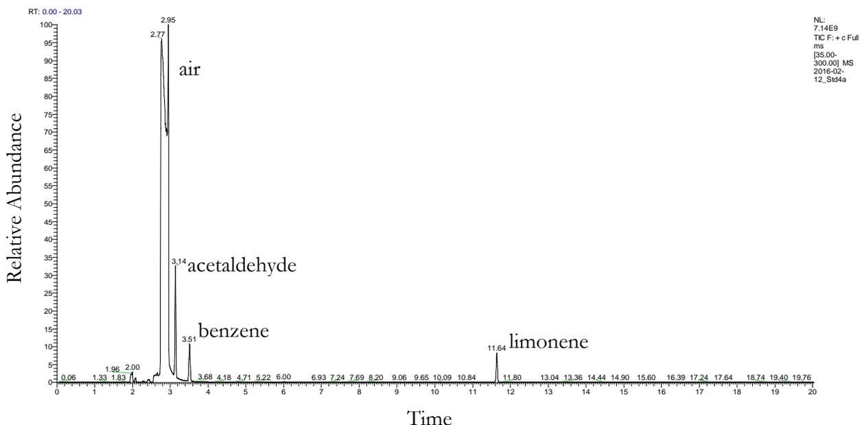
**Figure 4: Volatile components as measured using head space gas chromatography. (Acetaldehyde at 3.14 min, benzene at 3.51 min and limonene at 11.64 min)**
