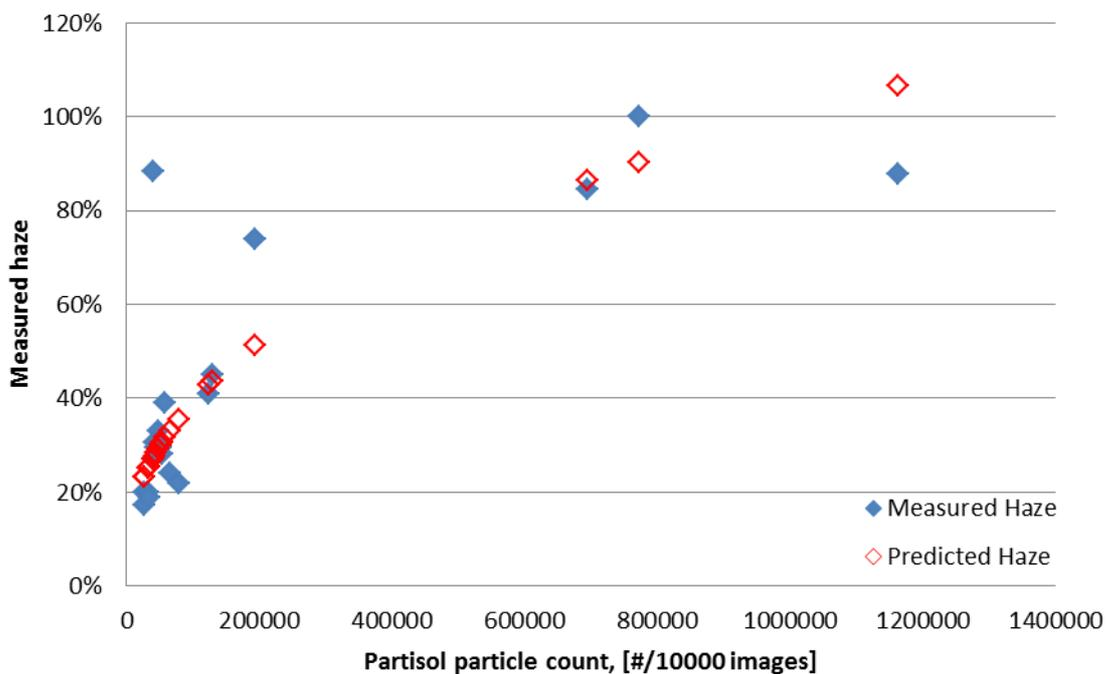
Figure 39: correlation between the measured haze values for the samples of task 2 and 3 and the measured partisol counts for the same samples.
