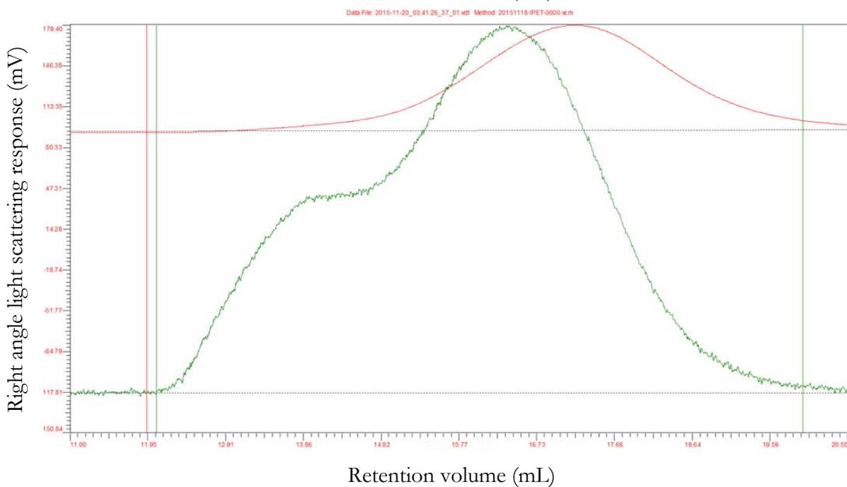
**Figure 20: Gel-partitioning chromatogram for normal rPET (above) and rPET to which EVOH is added (below). In GPC's the largest masses run first of the column and the smallest masses as last. Hence the broad shoulder on the left side indicates the presence of molecules with a high molar mass. Red line = refractive index response, [mV] Green line = Right angle light scattering response, [mV]**
