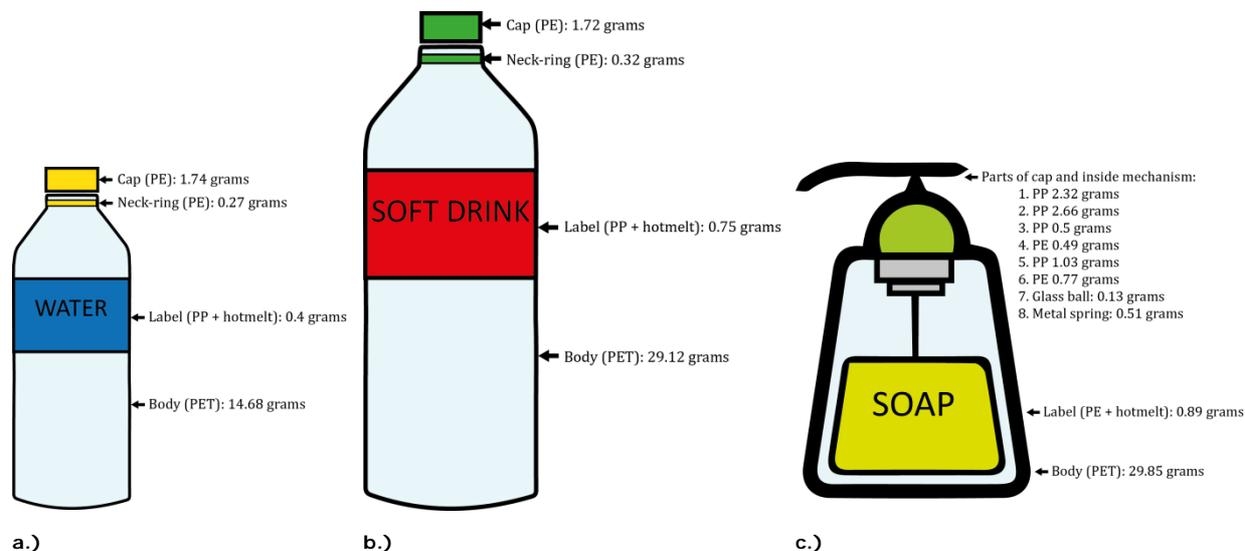
**Figure 7: The material composition of some typical PET bottles and flask. a.) typical transparent PET bottle 0.5 L. b.) typical transparent PET bottle 1.5 L c.) typical non-food soap flask with pump mechanism**
