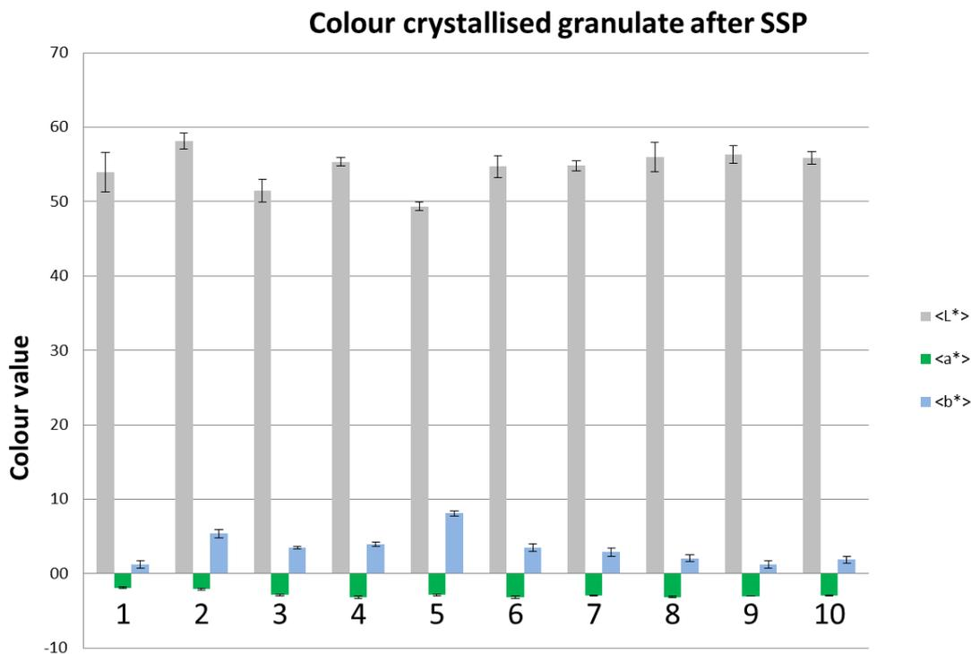
Figure 27: The CIELAB colour values for the crystallised granulates after SSP treatment.<sup>20</sup>
