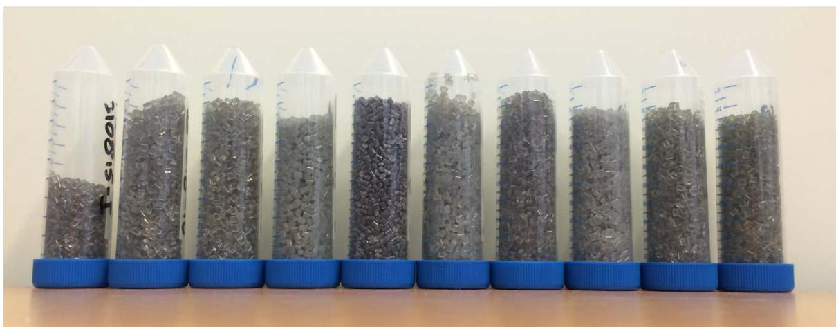
**Figure 14: Samples of the recycled PET granulates. Variations in the greyish colour caused by contaminants. From left to right: 0 rPET, 1 ink, 2 Amosorb, 3 PS, 4 PP, 5 PLA, 6 EVOH, 7 PE, 8 Nylon, 9 Hotmelt, 10 PVC.**
