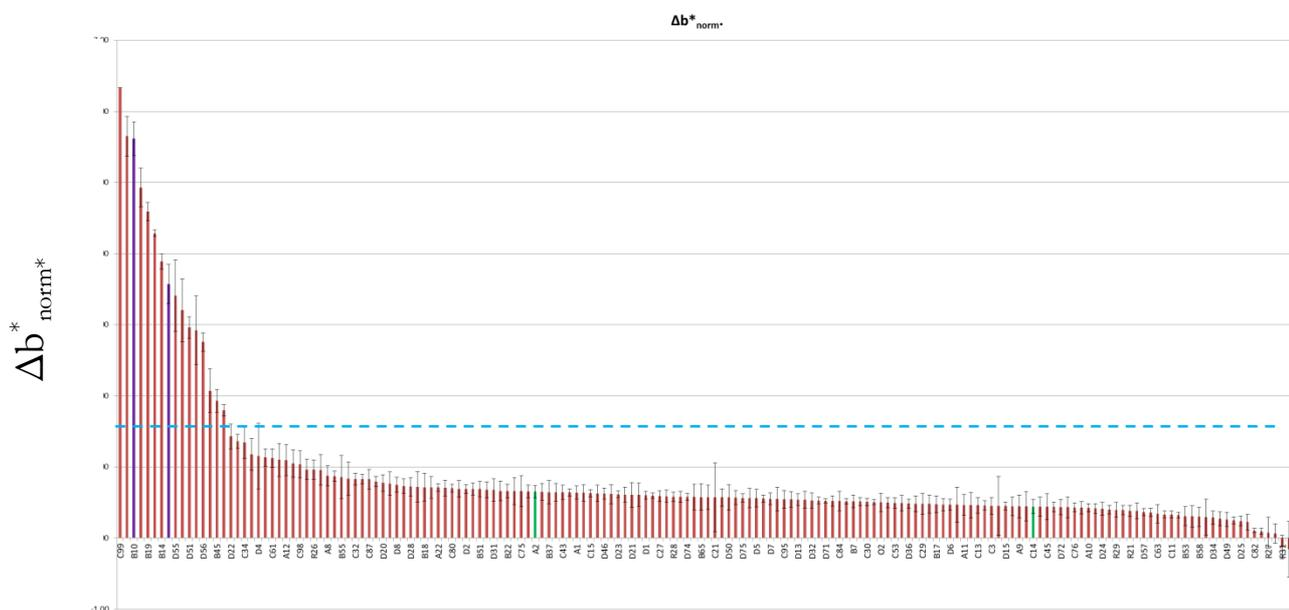
**Figure 8: The results of the barrier bottle identification test for 175 different bottles of the Dutch market. Displayed are the normalised differences in  $b^*$  colour value. The purple bars are for known barrier bottles, the green bars for known non-barrier bottles. The blue dashed line is the threshold value of 1.6.**
