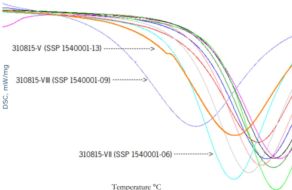
Figure 26: Superposition of the first heating run with DSC for all the samples in task 2 in the temperature range 100-130°C.
