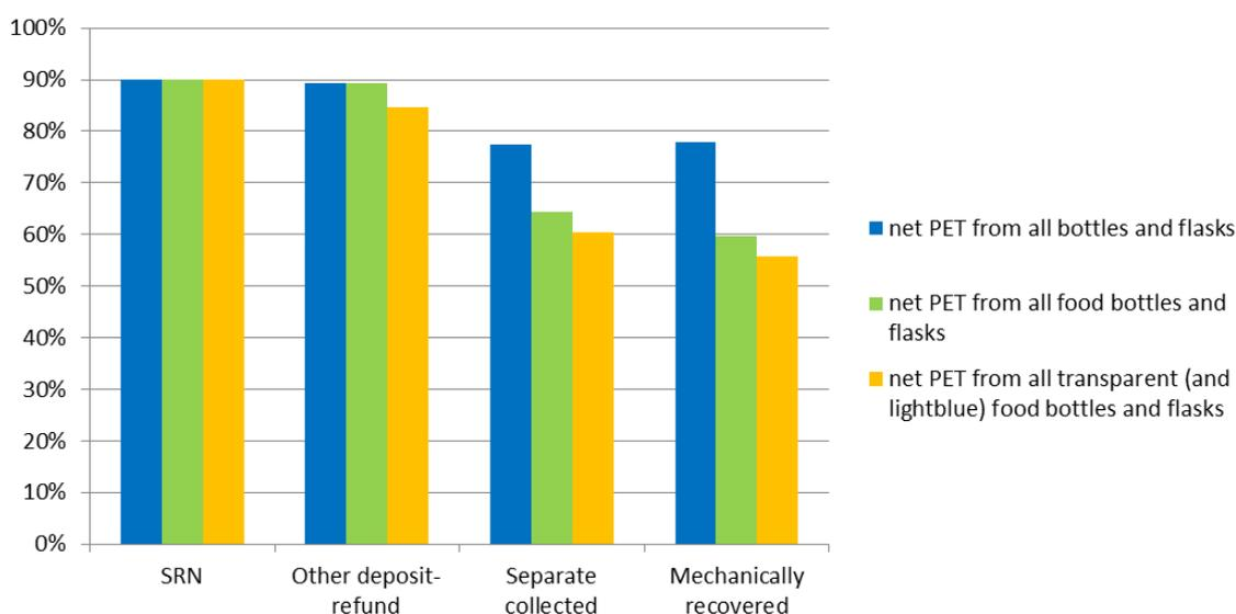
**Figure 11: The net PET material content of sorted PET products originating from three different collection systems in [% w dm/w dm].**
