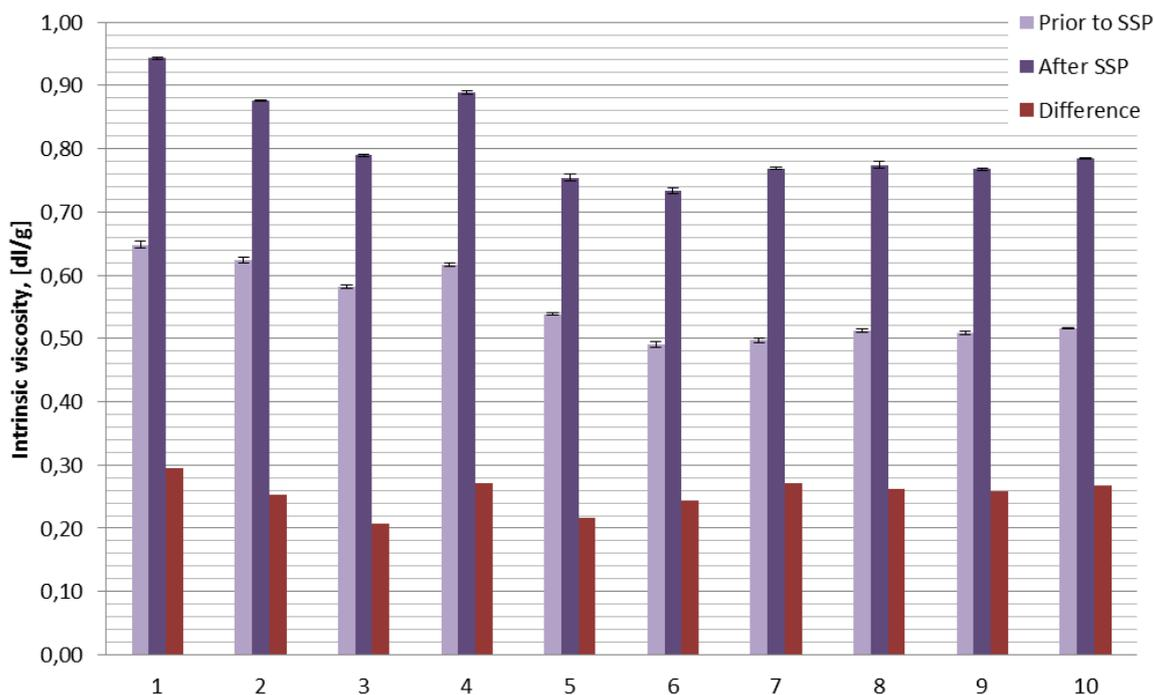
**Figure 30: The intrinsic viscosities of the ten combinations of feedstock and process before and after the SSP treatment.**
