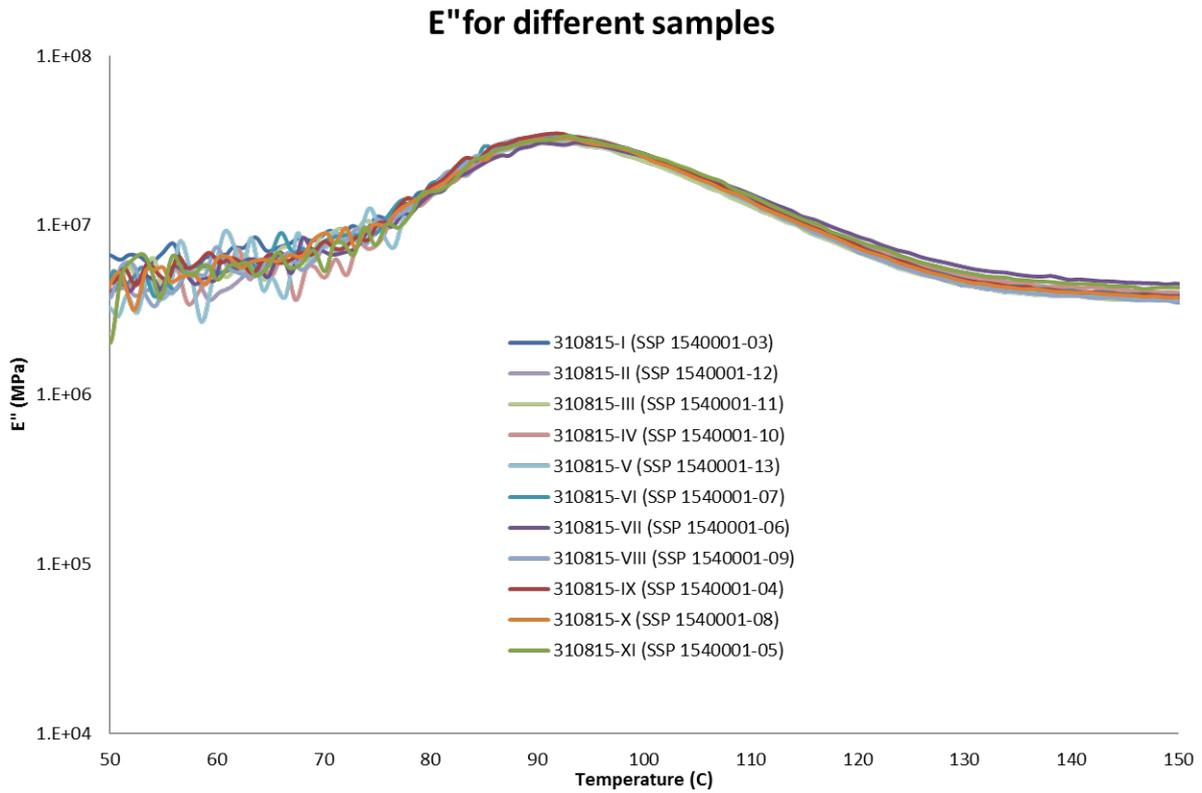
Figure 24: DMT-analysis of the loss moduli (E'') around the glass transition temperature of PET.
