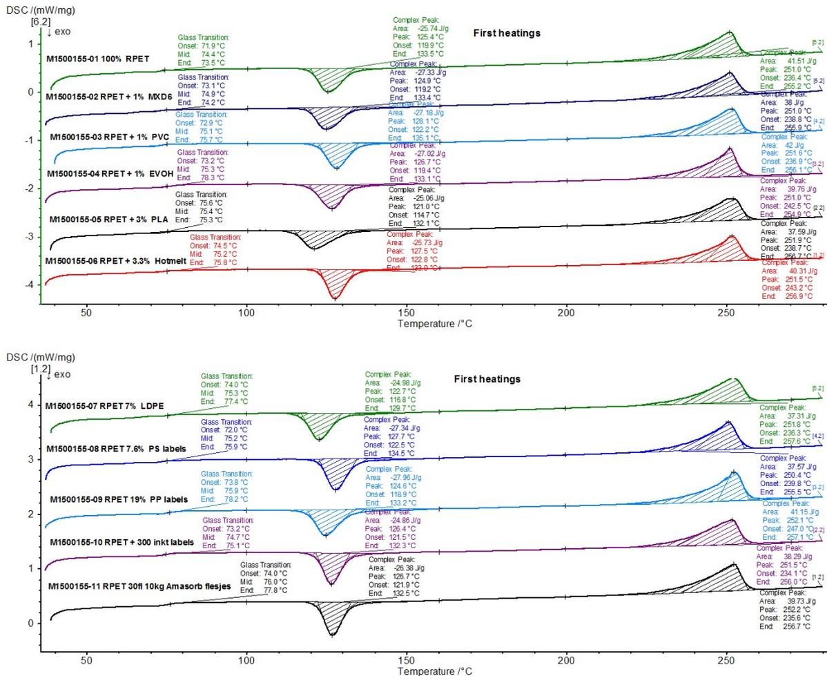
**Figure 21: Thermograms showing the first heating scans of the rPET and 10 deliberately contaminated rPET samples. DSC thermograms show the enthalpy that is released or absorbed during the heating scans.**
