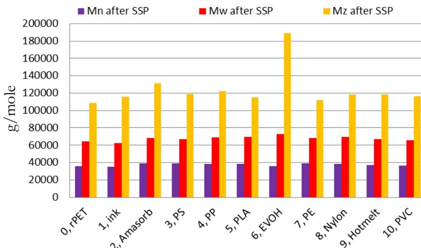
Figure 19: The three types of average molecular weights for the PET samples after SSP treatment.
