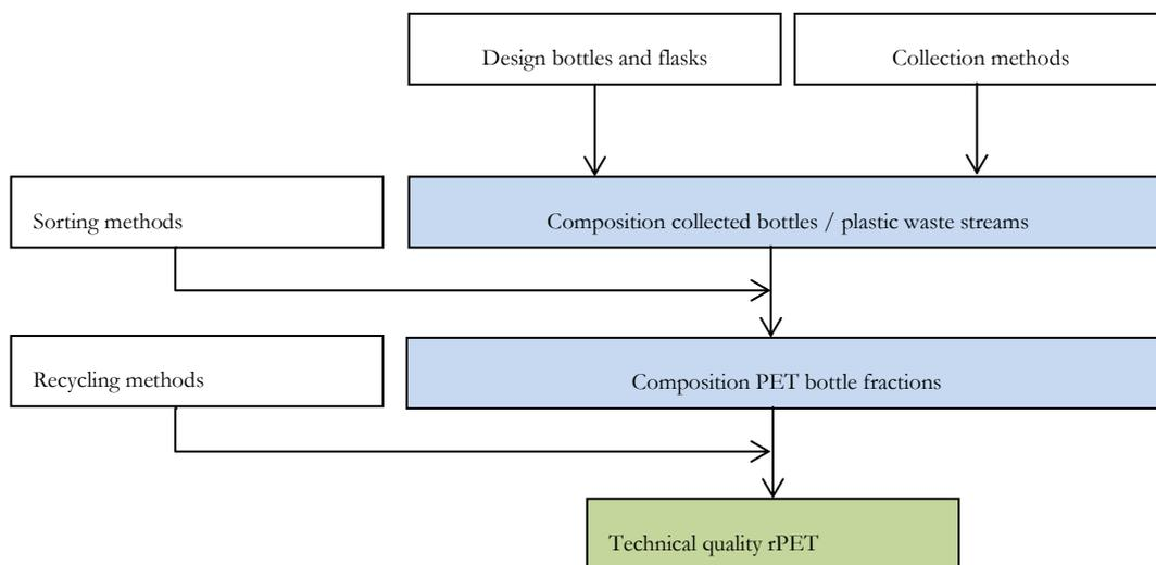
**Figure 1: The technical quality of the retrieved rPET is determined by a complex interaction between the bottle design, collection methods, sorting methods and recycling methods.**
