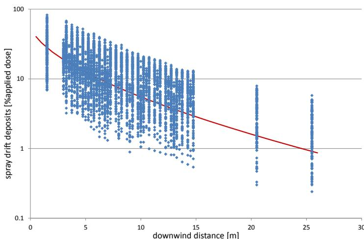
**Figure 1: Downwind deposits of spray drift as a function of distance, gathered for all experiments. Solid line: typical decay as a function of distance.**
