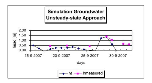
The simulations indicate that with the selected drain spacing the watertable indeed drops back to 0.90 m after 36 hours. Thus it can be concluded that the selected drain spacing are appropriate.
