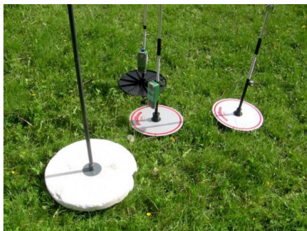
Figure 6.3 Grass height meters used at Dairy Campus for field measurements
