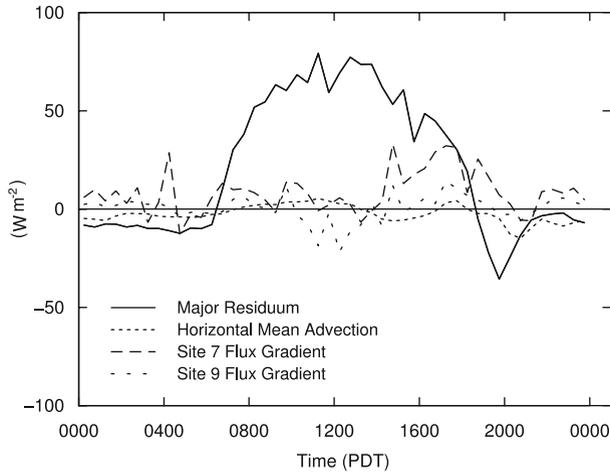
**Fig. 10** The diurnal composite of the mean horizontal advection of sensible heat along with the vertical sensible heat flux divergence calculated from direct measurements at sites 7 and 9. The residuum found from the major terms is shown for comparison. Positive values indicate heat accumulating near the surface
