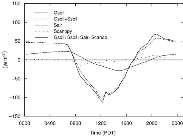
**Fig. 5** The diurnal composite over all sites and days of the total surface heating  $G$  and the various terms comprising it.  $G_{soil}$  is the heat flux measured by the heat flux plates at 50 mm depth,  $S_{soil}$  is the heat storage in the soil above the heat flux plate,  $S_{canopy}$  is the heat storage by the above-ground plant biomass, and  $S_{air}$  is the heat storage by air in the canopy. Note that  $S_{air}$  is undistinguishable from the reference line at 0
