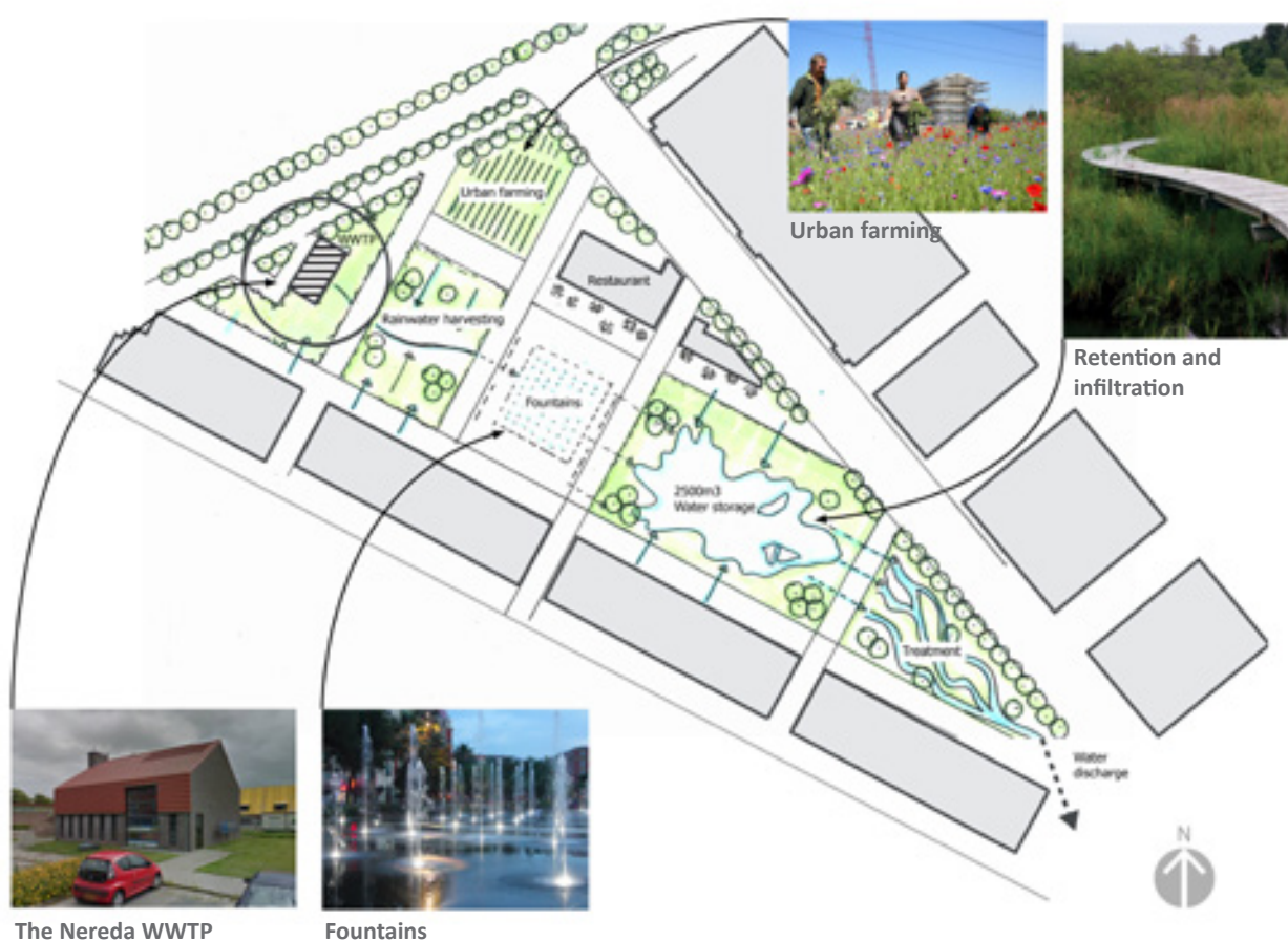
Figure 4.8 The Nereda® model (model A)
