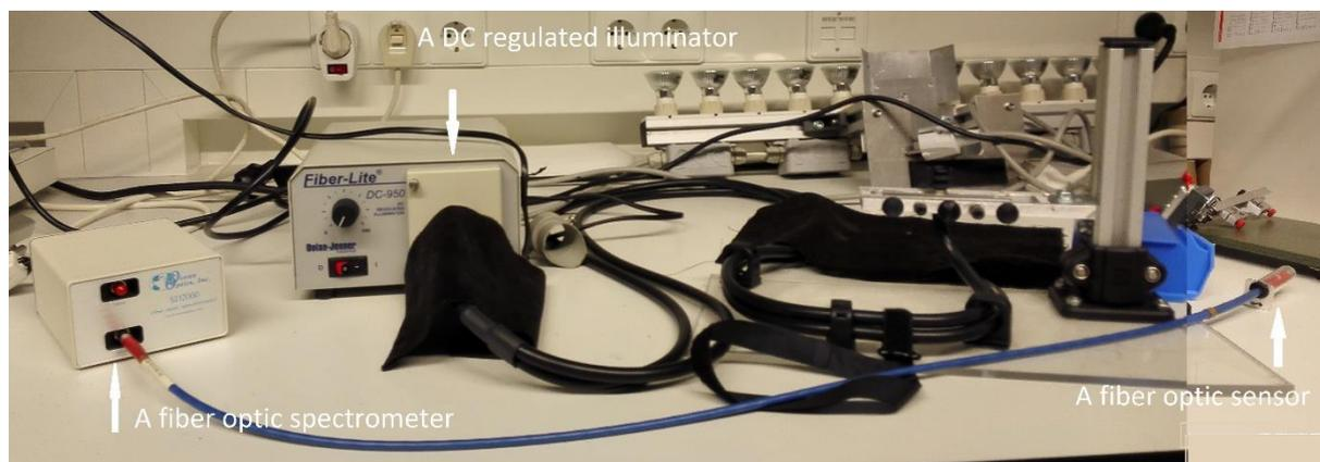
Figure A4. The composition of VIS-NIR transmittance system.
