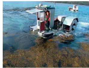
c) Vessel with a paddle wheel cutter, used to harvest Ascophyllum nodosum in Norway © Sander.
