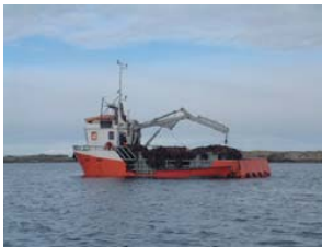
a) Vessel with seaweed trawl, used to harvest Laminaria hyperborea in Norway © FMC biopolymer Corp.
