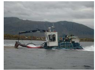
d) Vessel with a vaccum-sucker, used to harvest Ascophyllum nodosum in Norway © Rebours.
