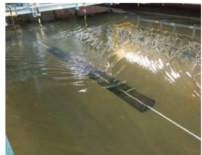
Figure 8-11: Impression of model test of the Ulva Cage. The Ulva is contained within the cage of 4.8 x D0.3 m.
