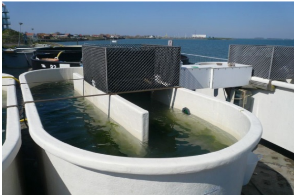
Figure 6-1 Six raceways and six tanks that were continuously supplied with running Oosterschelde water (no nutrients added) were used for the Ulva experiments
