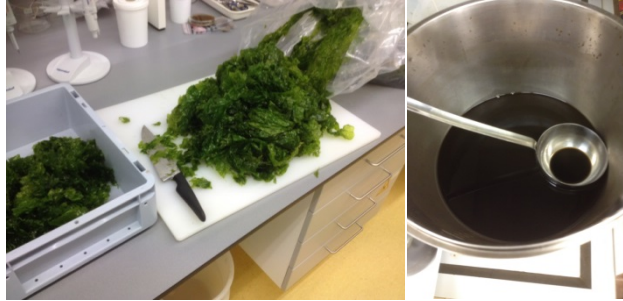
Figure 9-8 Ulva feedstock (left) and process product from hydrolysis at 140 °C (run 1, right).
