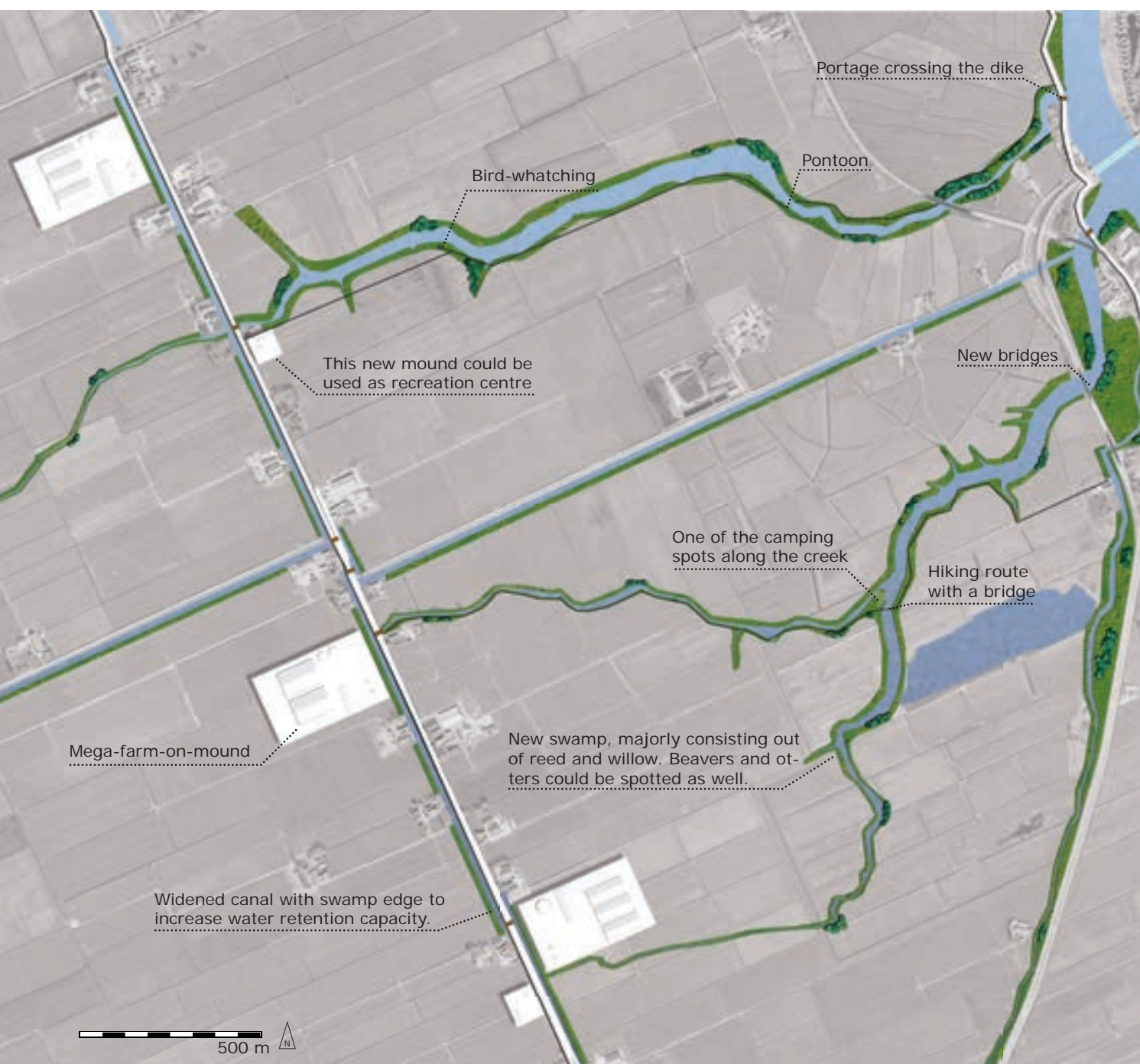
Figure 5.8 | The natural shaped creek system contrast with the rectangular shaped new mounds and compartmentdikes.
