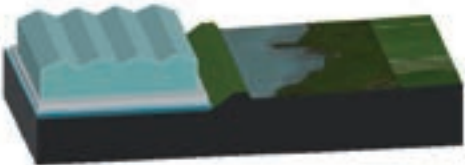
Figure 4.4C | The solution: floating greenhouses in the Koekoekspolder, and a swamp zone around, reducing seepage.
