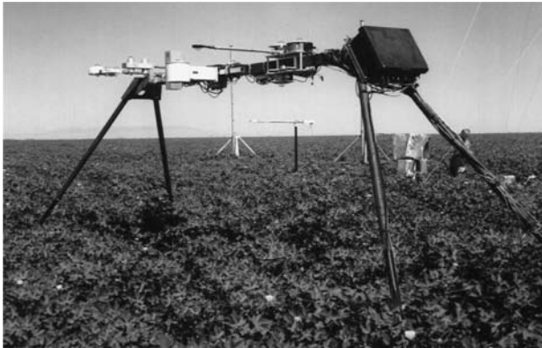
Fig. 1 The radiation instrumentation (“dark horse”) at site 7. In the background, in the middle can be seen the Schulze–Däke net radiometer
