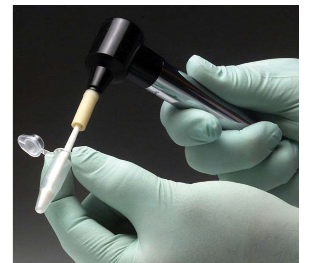
Figure 3. Disposable micro-potter with battery-driven hand-held rotor for homogenisation of bulb tissue in extraction buffer.
