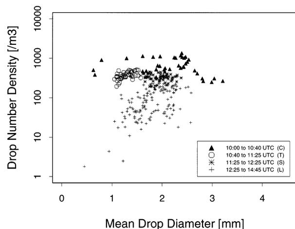
FIG. 8. Variability of the raindrop size distribution for the distinct phases of the 27 May 1997 squall line storm (Fig. 5), as reflected by the mass-weighted mean drop size  $\bar{D}_m$  and drop number density  $N_T$ .
