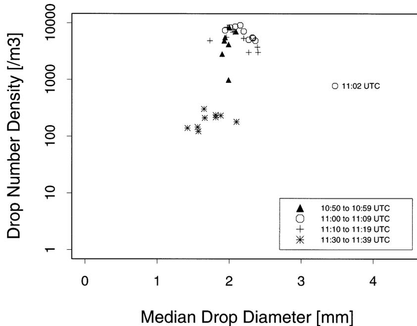
FIG. 4. Variability of the raindrop size distribution of the 21 Jun 1958 storm near Miami, FL, as reflected by the median drop size  $D_0$  and drop number density  $N_T$ . Four 10-min periods are distinguished.
