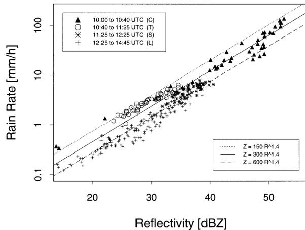
FIG. 6. Variability of the  $Z$ - $R$  relationship between distinct phases of the 27 May 1997 squall line storm (Fig. 5), as reflected by the raindrop spectra data collected using a Joss-Waldvogel (1967) disdrometer in Goodwin Creek, northern MS. [Adapted from Steiner et al. (1999).]
