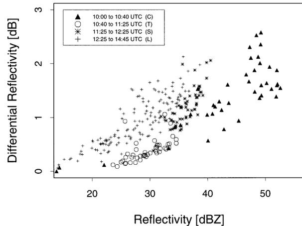
FIG. 7. Variability of the raindrop size distribution for the distinct phases of the 27 May 1997 squall line storm (Fig. 5), as reflected by the radar reflectivity factor  $Z$  and differential reflectivity  $Z_{DR}$ .
