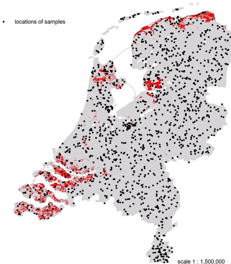
Fig. 1. Locations of the national stratified soil survey sampling (Finke et al., 2001). The red area is an example of the location of one of the 95 strata (calcareous silty clay soils with a MHW between 0.4 and 0.8 m) that is distinguished in the national stratified soil survey.
