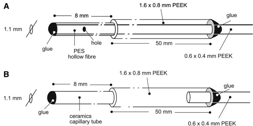
resistance. This 0.6 mm PEEK tube inside the PES fibre had a 0.1 mm hole in the centre to connect the PES lumen with the 1.6 mm PEEK tube lumen. The ceramic samplers (Fig. 1B) had 50 mm 0.6 mm PEEK glued in the backside of the 50 mm long 1.6 mm PEEK.
