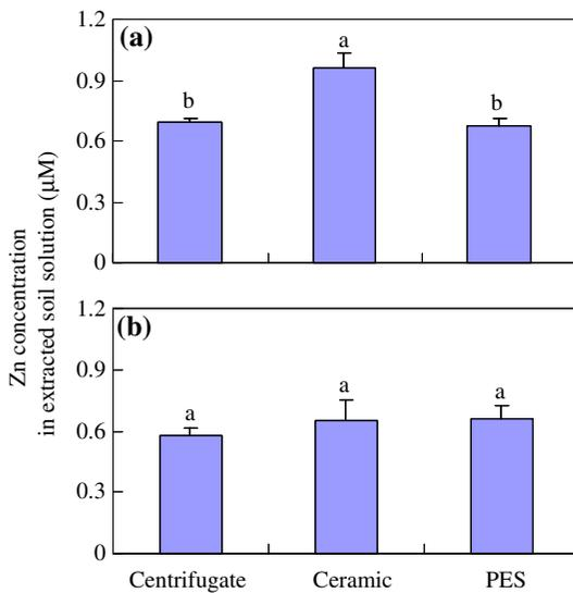
**Fig. 5** Zn concentrations in a soil solution collected by centrifugation, or by micro-pore-water samplers with ceramic or PES cups. A sandy soil was mixed with a 0.2  $\mu\text{M}$  (a) or 15  $\mu\text{M}$   $\text{Zn}(\text{NO}_3)_2$  solution (b), and packed into rhizotrons. Results for the cups are means of three replicates. Vertical bars represent  $\pm$  SE ( $n = 3$ ). The data with the different letters show significant difference among treatments at  $P < 0.05$
