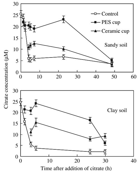
**Fig. 2** Change in citrate concentration with time in a proxy of a soil solution stored as such (control), or stored after passing the PES or ceramic suction cups. At  $t = 0$  h citrate was added to the soil solution. Sampling took about 1.3 h for PES cups and about 4 h for ceramic cups. Results are means of three replicates for each vertical bars represent  $\pm$  SE ( $n = 3$ )
