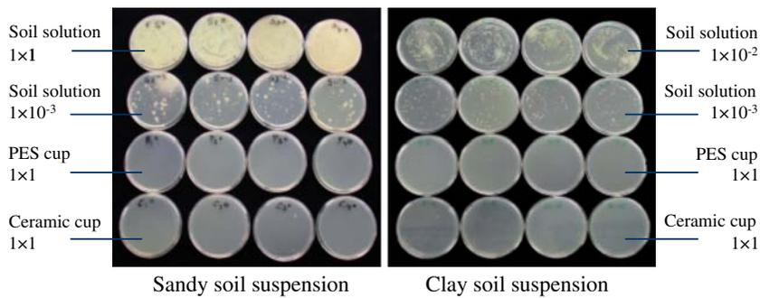
**Fig. 3** Effect of micro-suction cups on filtering microorganism in collecting soil or rhizosphere solution in sandy or clay soils. The original soil solution was prepared with demineralized water ( $2 \text{ ml g}^{-1}$  soil). “ $1 \times 1$ ” indicates
