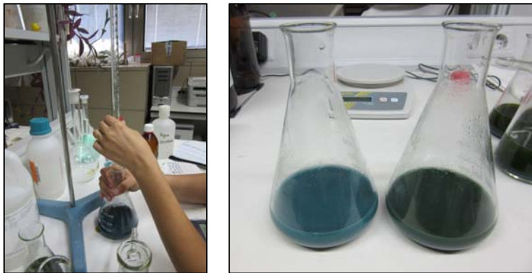
Figure 5: a) The SOC determination by manual titration and b) the colour change from blue to green.
