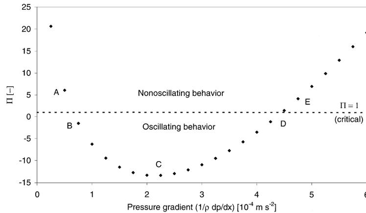
FIG. 2. The dimensionless intermittency parameter  $\Pi$  as a function of the pressure gradient. The critical level  $\Pi = 1$ , which separates two different types of system behavior, is given by the small dotted line.
