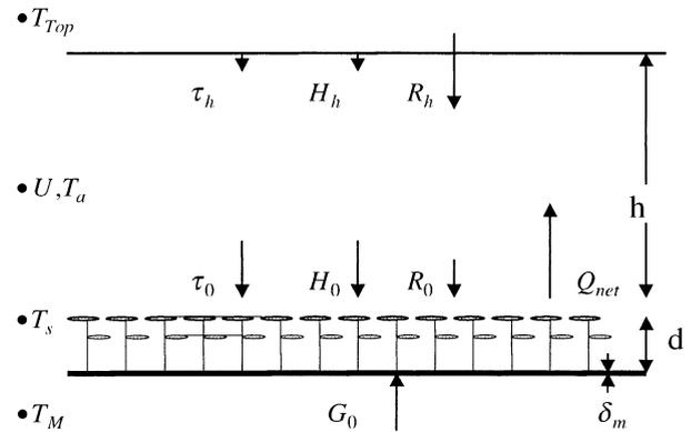
FIG. 1. An overview of the model system: state variables, fluxes, and model domain. The symbols are explained in appendix A. A detailed system description is given in Part I.
