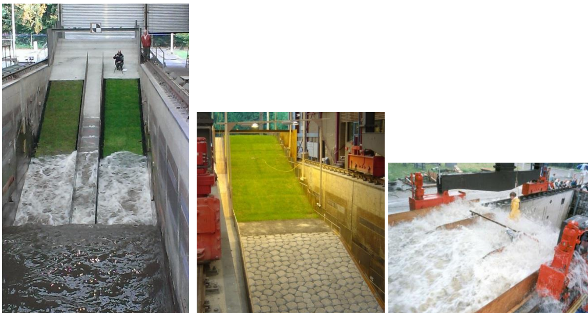
Figure 2.9 Large scale wave flume research in the Deltares Delta Flume. Left: wave run-up. Middle: test set-up prior to testing. Right: overtopping while a (secured) person was standing on the crest.
