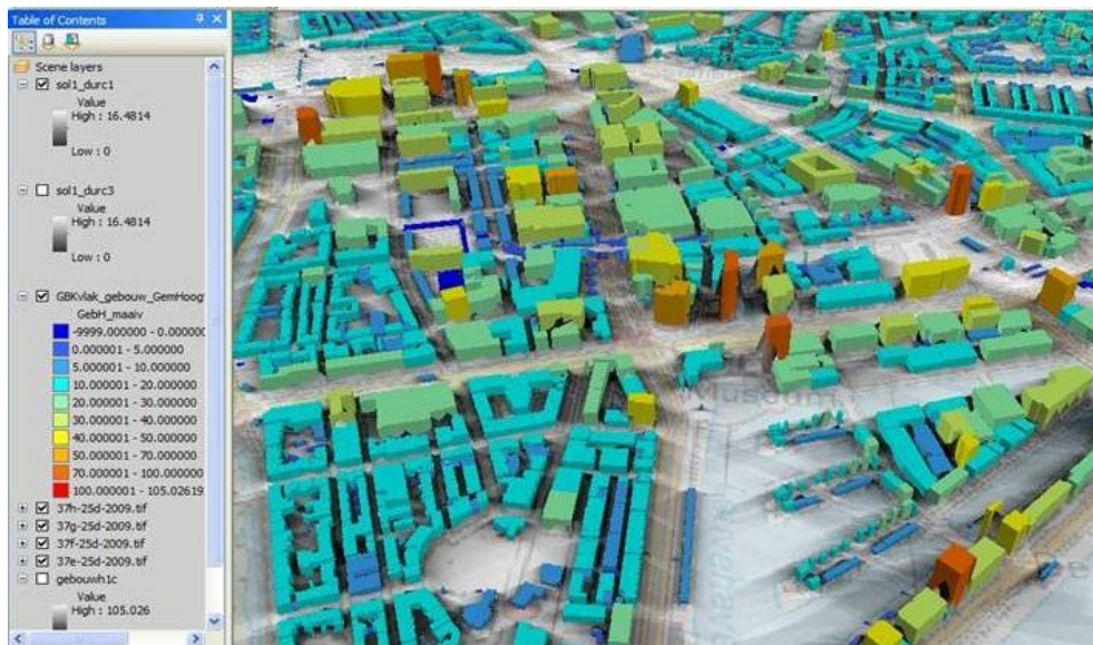
Figure 35 Detailed view of the shade due to buildings in Rotterdam.
