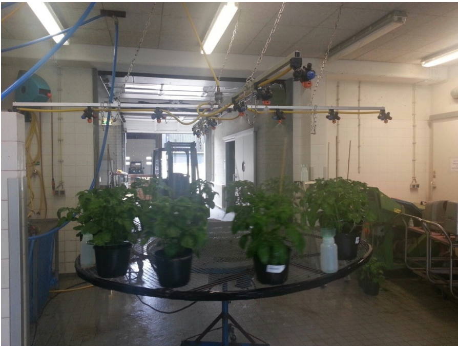
Figure 2.2. Rain simulation with 36 mm of tap water in a period of 15 minutes.
