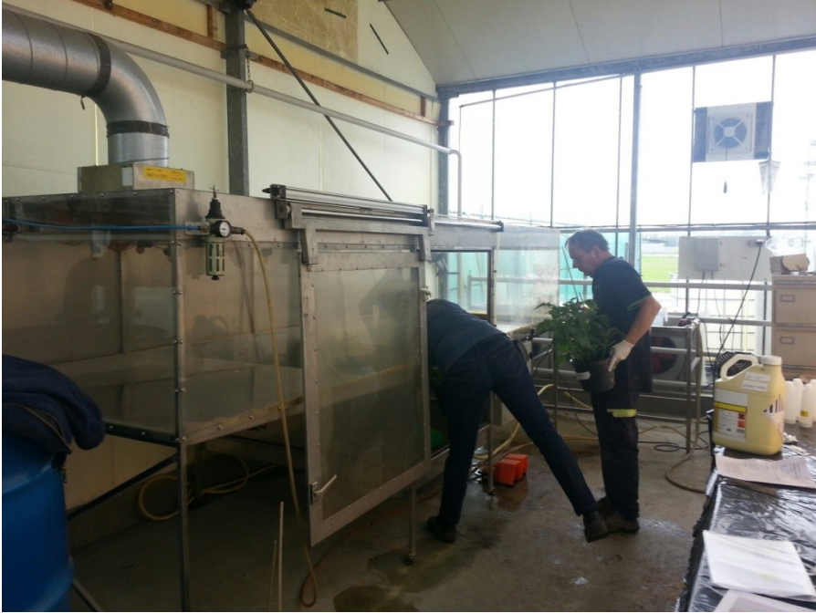
Figure 2.1. Spray cabine at PPO Lelystad used to spray the plants.
