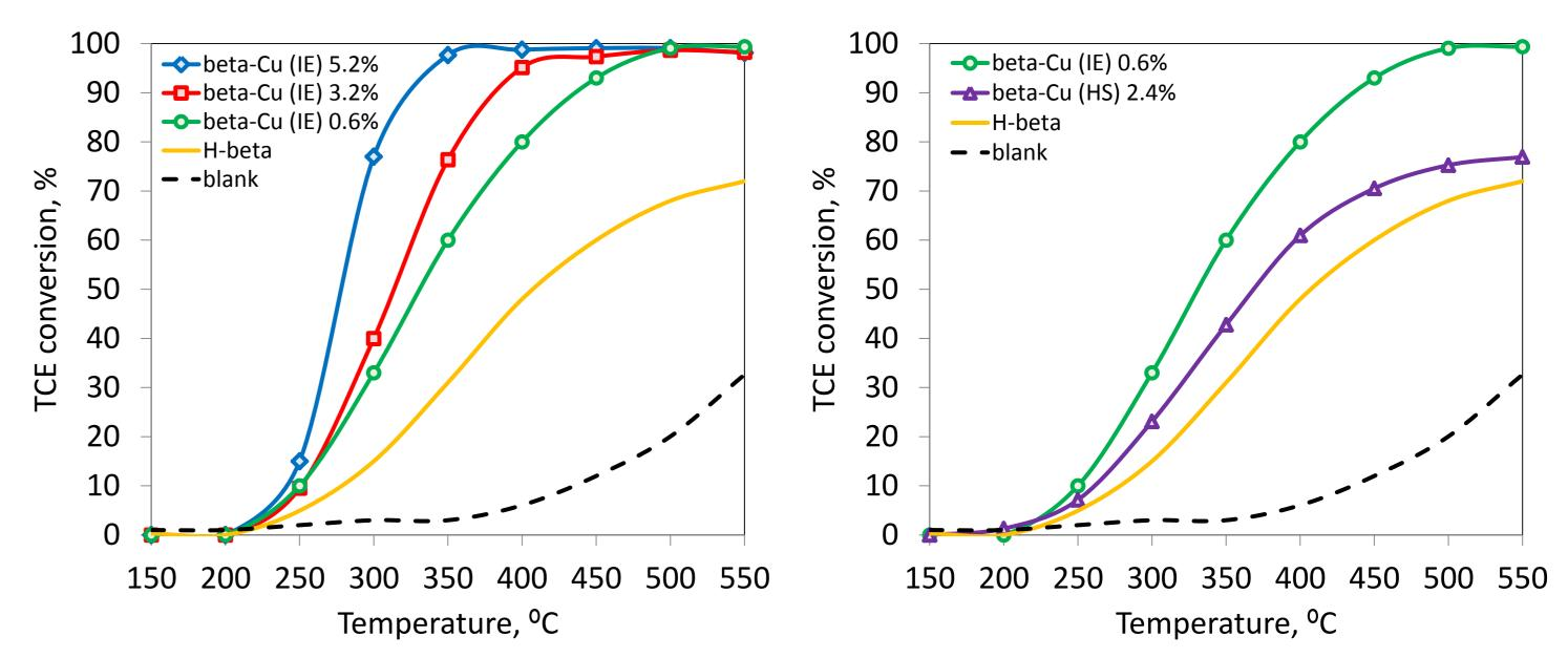
The increasing addition of Cu (0.6, 3.2 and 5.2%wt) decreases the T<sub>50</sub> (330, 310 and 275°C, respectively).
