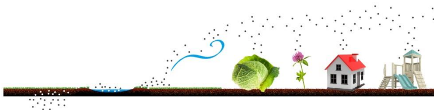
Figure I. Source: contaminated soil. Path: from soil to surface water, next to sediment and next resuspension via wind erosion into the air. Receptor: surface water, atmospheric deposition of POPs containing particles in e.g. vegetables, houses, flowers and playgrounds.
