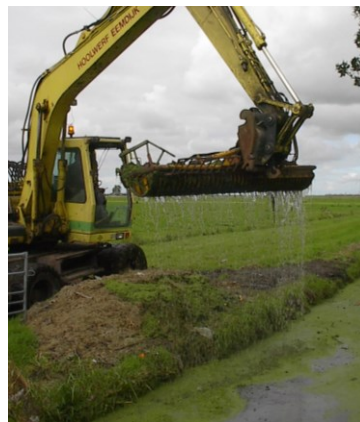
Figure 2 Harvesting duckweed from a creek with a dredge covered with fine gauze.
