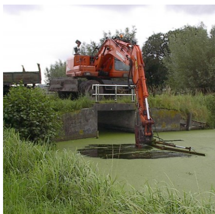
Figure 1 Harvesting duckweed from a creek with a flat sieve pan.
