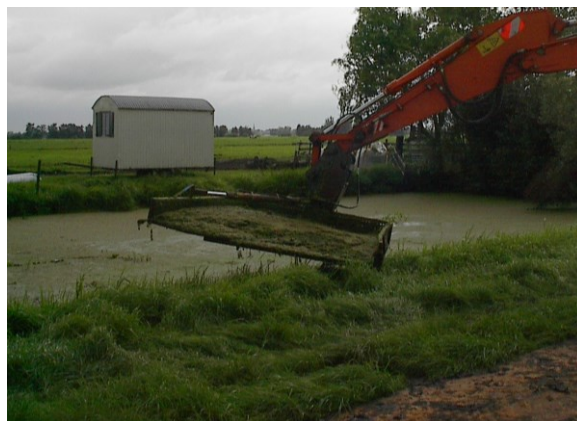
Figure 1 Harvesting duckweed from a creek with a flat sieve pan.
