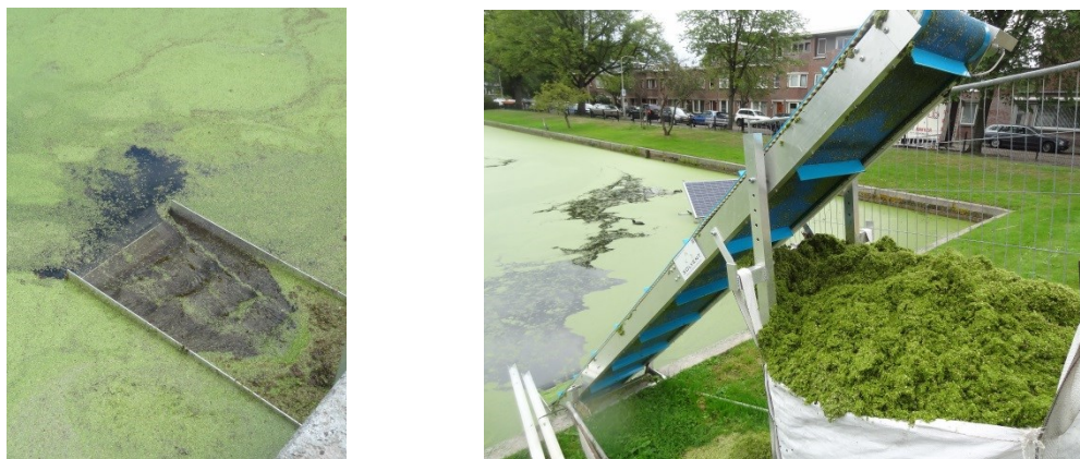
Figure 4 Harvesting duckweed with the Duckweed Guzzler and Belt (Bom Aqua B.V.).
