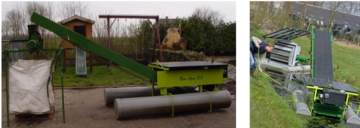
Figure 3 Harvesting duckweed from a creek with an automatic solar-powered conveyor belt.
