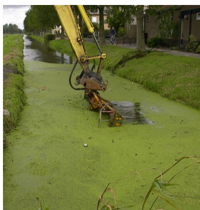
Figure 2 Harvesting duckweed from a creek with a dredge covered with fine gauze.
