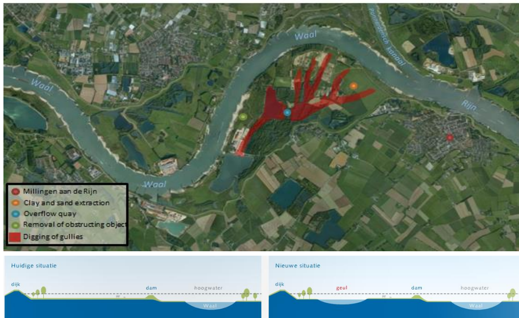
Figure 8. Graphic representation of the current measures in the Ooijpolder. The lower left illustrates the current situation and the lower right illustrates the new situation where the gullies have been dug. Based on infographic from R. v. d. Rivier (2015) and maps (2015).
