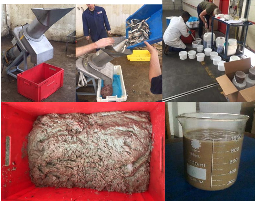
Figure 5. The process of fish silage production from sardines.
