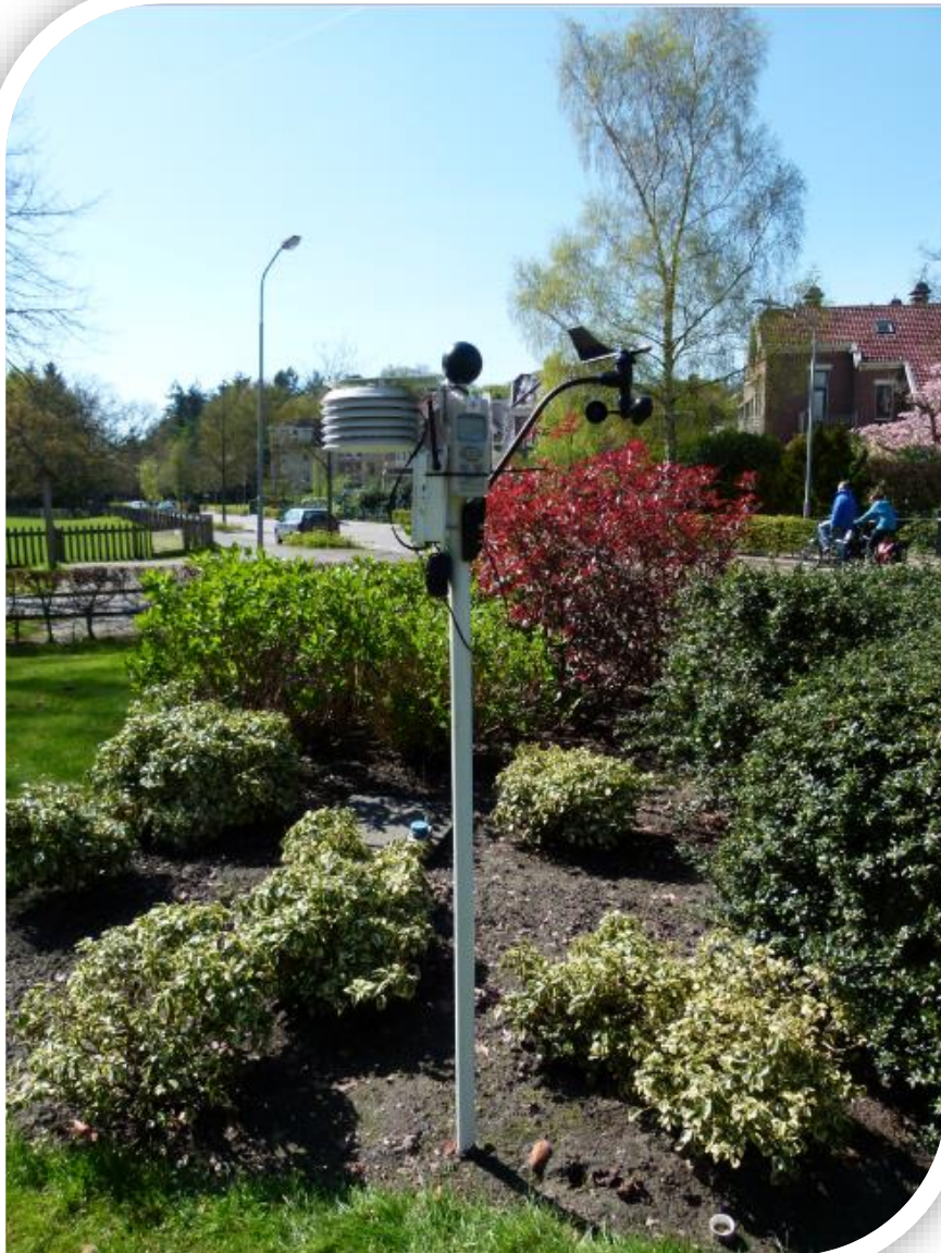
Weather station equipped with temperature and humidity sensors, anemometer and globe thermometer at INCAS 3 , Assen (latitude: 53° 0' 0'' N, longitude of 6° 55' 00'' E).
