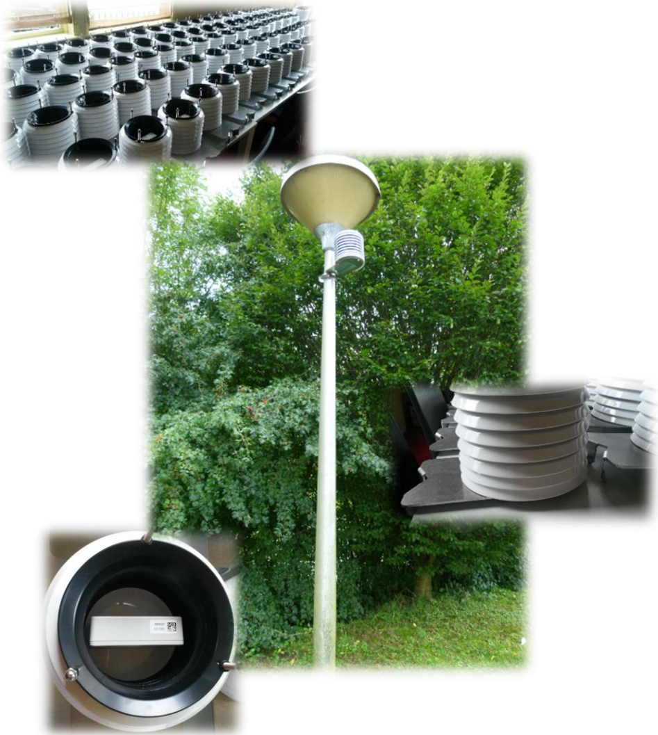
An example of 100 wireless sensor nodes equipped with air temperature and humidity sensors at the Zernike Campus, Groningen (latitude: 53°24' 0'' N, longitude of 6° 53' 00'' E).
