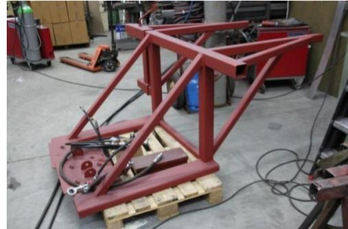
Picture 14 Frame for transport of modules
