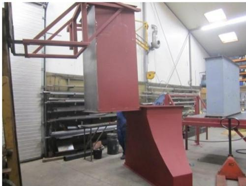
Picture 17. Placing upper box on transition
