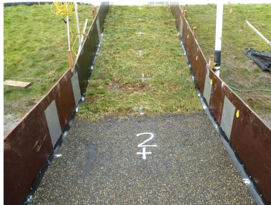
Figure 5.4. Slight erosion at the transition to the upper slope, test 2
