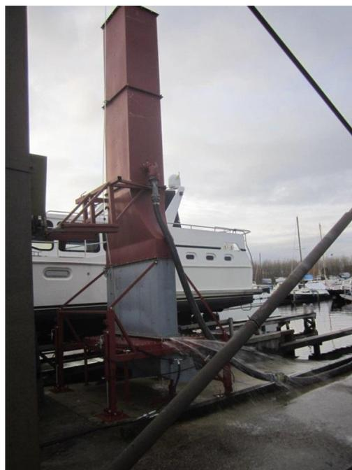
Picture 32. Testing with 7 m water column
