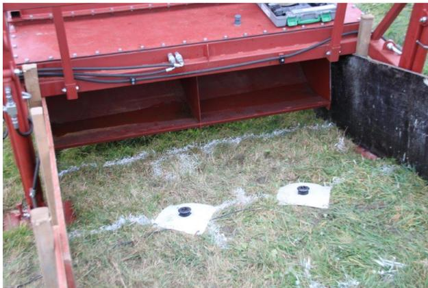
Figure 7. First two paddle wheels 3 cm above soil
