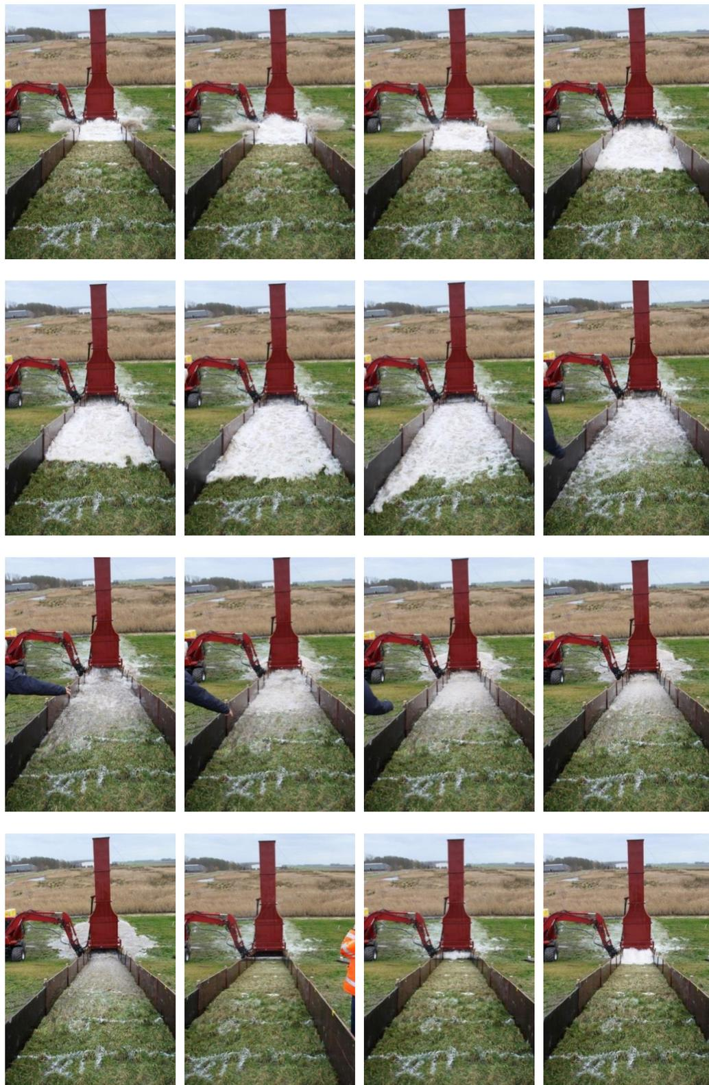
Figure 12. The run-up process for a filling level of 6 m.
