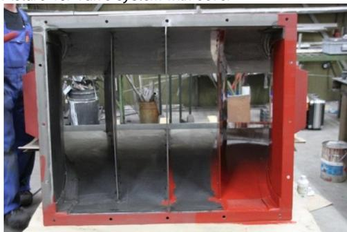
Picture 12. Inner part with guiding plates
