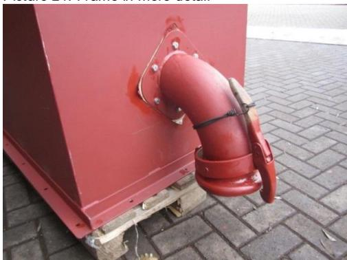
Picture 23. Inlet for pump on upper module
