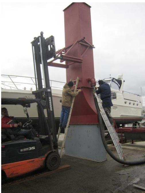
Picture 31. Fixing for 7 m water column testing
