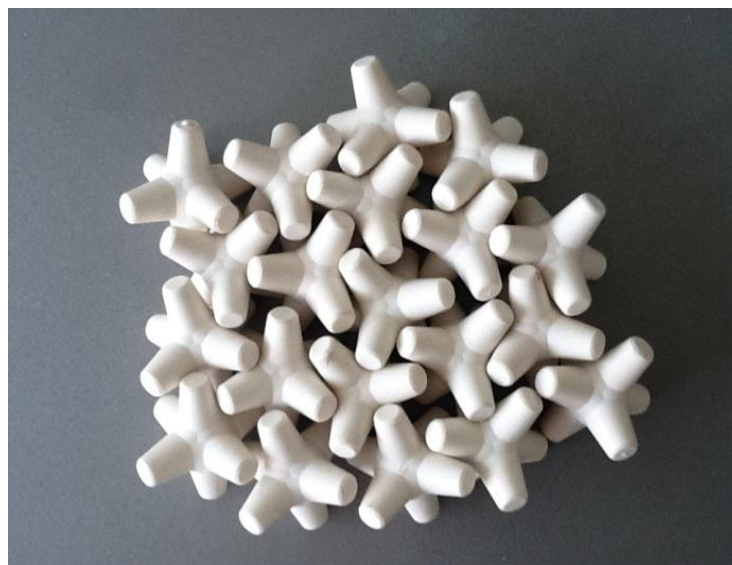
Figure 2.7 Random placement of crablock [Source: Hendrikse and Heijboer (2014)]
