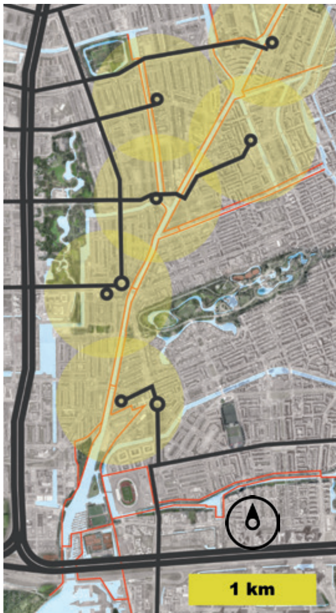
Figure 8.27: The circles with a radius of 500 metres indicates the range of the parking garages connected to the main roads
