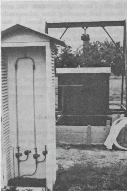
Fig. 2 Lysimeter during construction; manometer on the left, lysimeter tank above cellar in the background.
