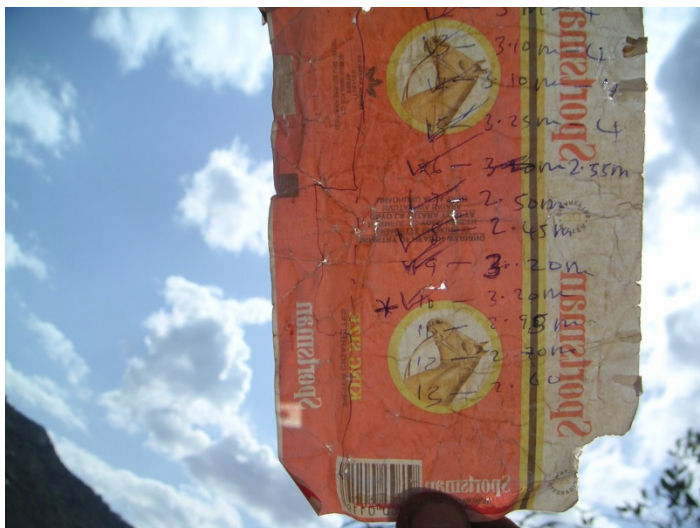
Figure 28 A package of "Sportsman" cigarettes folded open. The design of a sand dam and its measurements hand written on it
