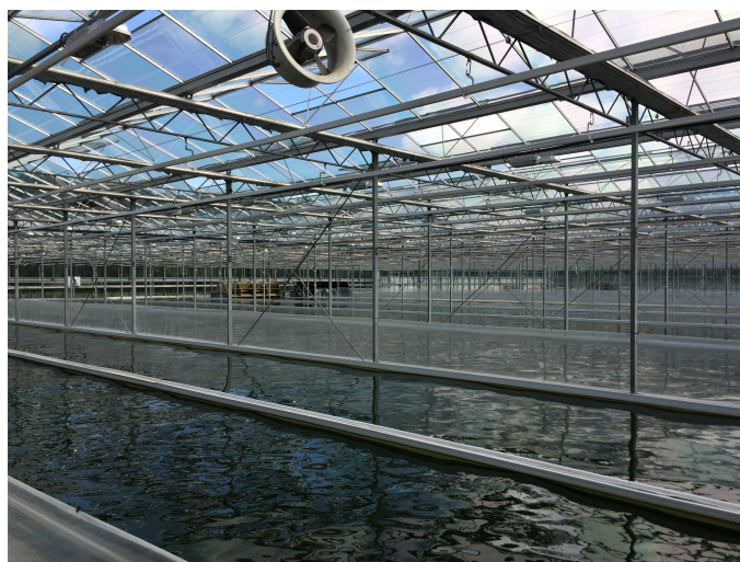
Figure 2-4: Raceway system in a greenhouse operated by Algaspring (Netherlands)
