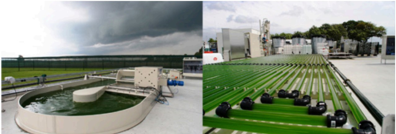
Figure 3-1. The two algae production systems operated at the research facility AlgaePARC at WUR. From left to right: (1) Raceway Pond; (2) Horizontal tubular PBR;
