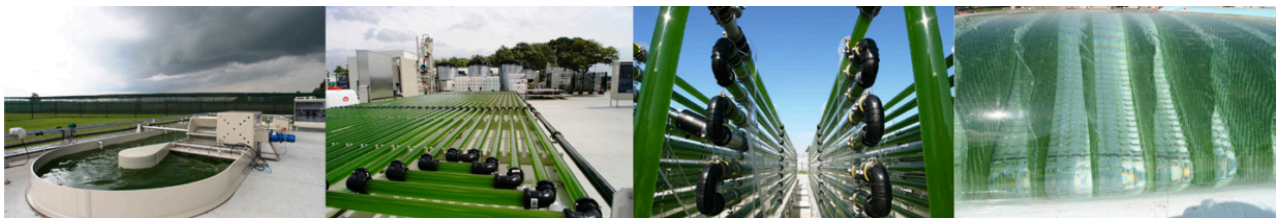
Figure 1-1. Four different algae production systems operated at the research facility AlgaePARC at WUR. From left to right: (1) Raceway Pond; (2) Horizontal tubular PBR; (3) Vertical stacked tubular PBR; (4) and Flat panel PBR [12].
