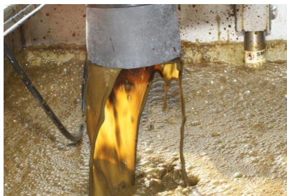
Figure 25. Liquid fraction flowing out of the separator.
