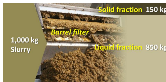
Figure 26. Slurry separation with a barrel filter.
