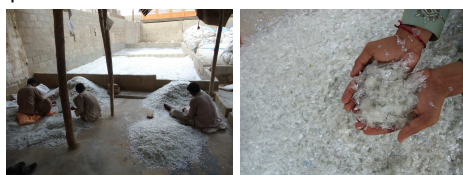
Figure 3 and 4: Sorting of grinded PET bottles on impurities in Pakistan.
