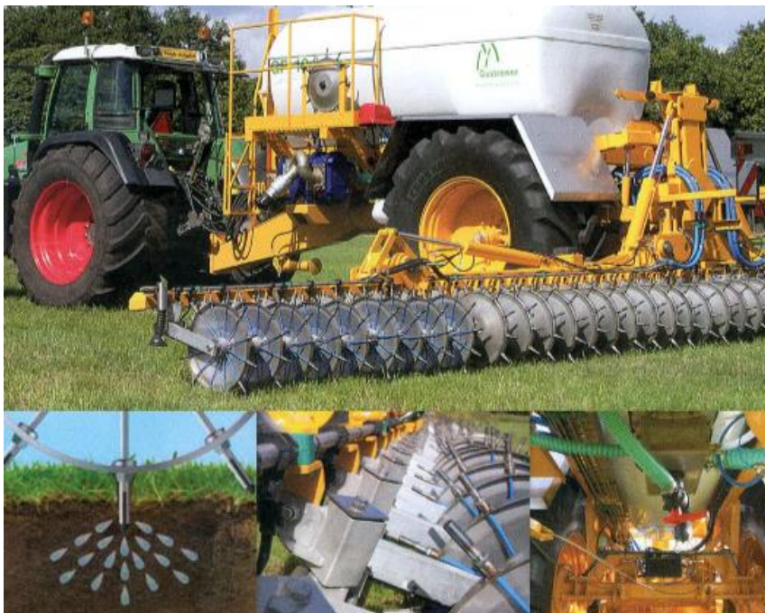
Figure 9: Spoked-wheel fertilizer (Gemeren, 2015)
