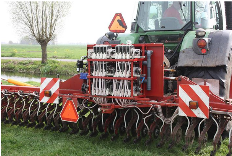
Figure 7: Disc injection fertilizer (Boerenbusiness, 2014)
